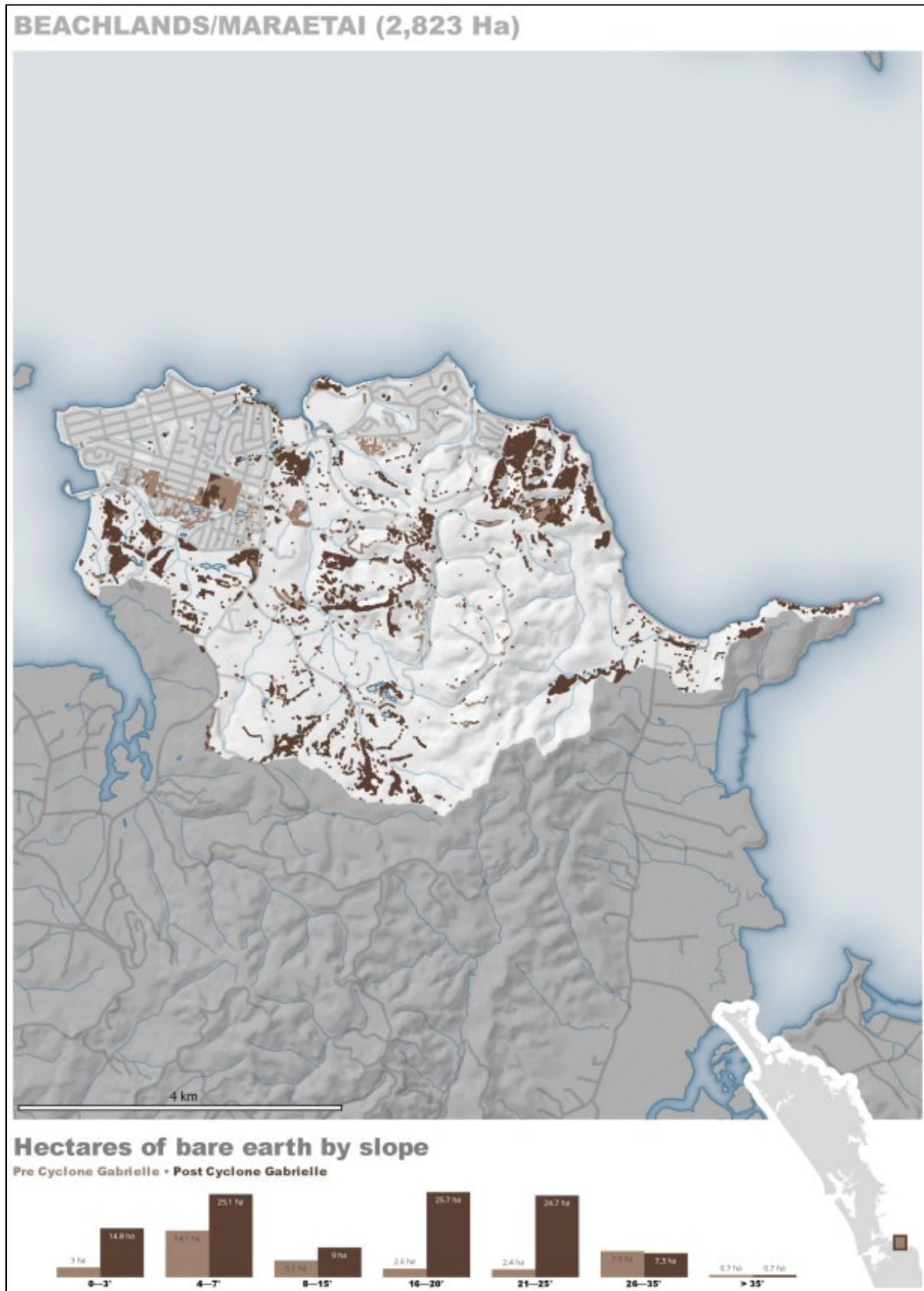
Figure 26: Pre- and post-Cyclone Gabrielle bare earth area (ha) by slope in the Beachlands/Maraetai catchment.
