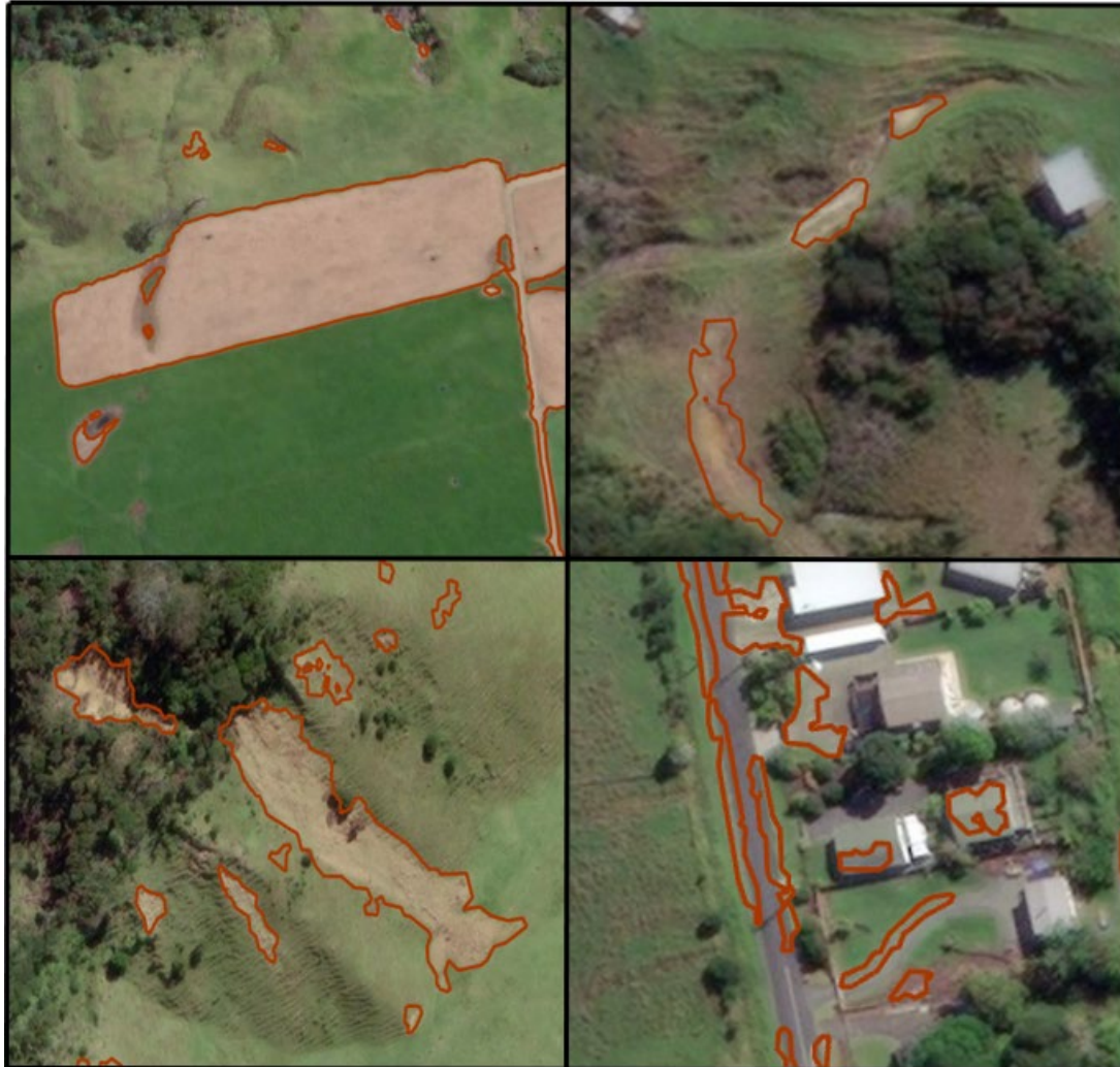
Figure 4: Inference output examples of bare earth, including false positives (bottom right panel).
