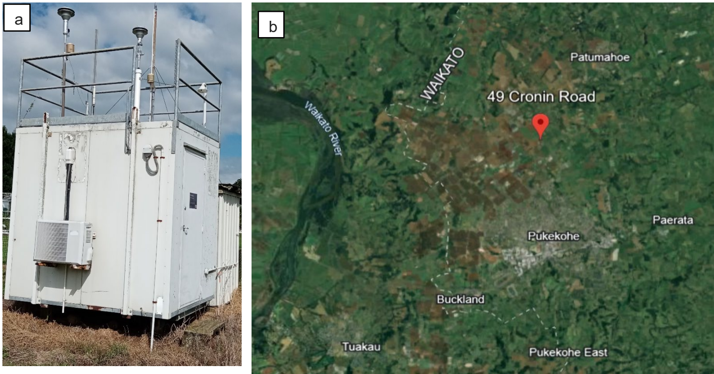
Figure 5. The Patumahoe air quality monitoring site is located within the Plant and Food Research Station at Cronin Rd, Patumahoe. Image ‘a’ shows the air quality monitoring shed. Image b is an aerial view of the monitoring site and surroundings taken in April 2024 (Source: Google Earth). Air quality monitoring at this site commenced on 21 October 1996. PM 10 , PM 2.5 , NO 2 , and ground level ozone concentrations are monitored at this site. This site represents Auckland regional background air quality. The main sources of air contaminants are motor vehicles, home heating, and agricultural activities such as fertiliser application, crop tilling and green waste burning.
