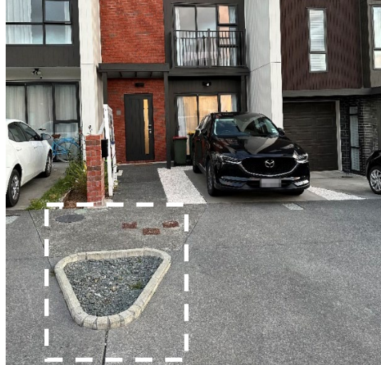
Figure 21: Grass was replaced with stones to improve access to parked car, and second car parks across footpath and planter space (as indicated by dashed white box)
