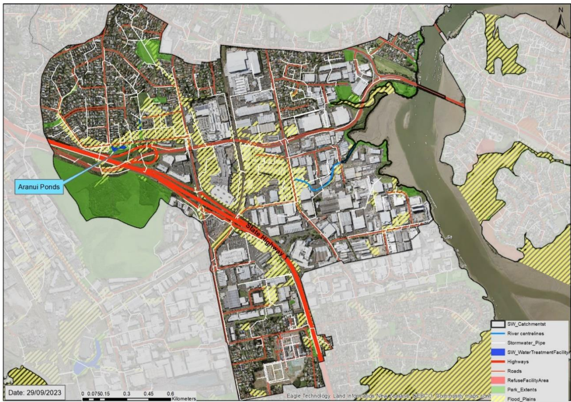
Figure 3. Zoomed-in view of Aranui stormwater treatment facility, showing the proximity of major roadways, nearby greenspace, the stormwater pipe network, flood plains, and the stormwater catchment boundary.
