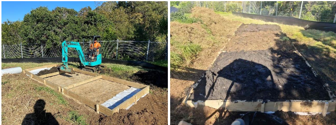
Figure 11. Portland Road, May 2022. establishing the trial plots. The plot with site-won topsoil is the middle of the three plots, with the darker plots on each side containing sediment.
