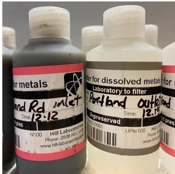
Figure 24. Samples of inlet to geobags before flocculation (left bottle), and leachate from geobags after flocculation (right bottle).
