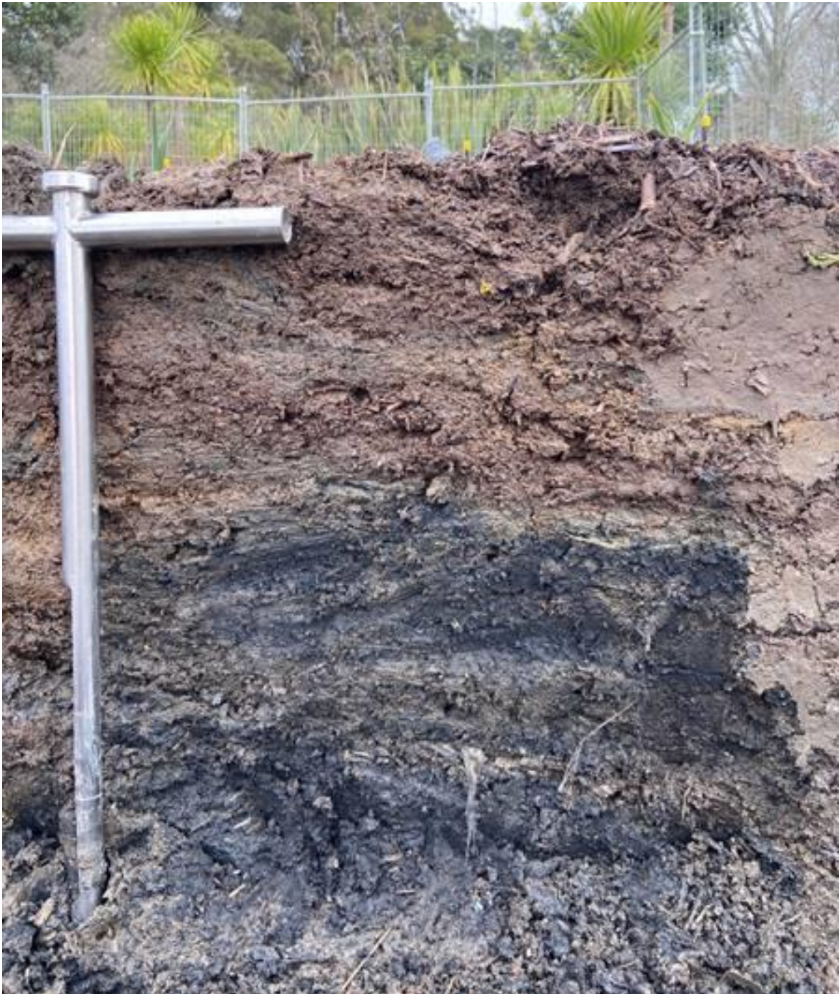
Figure 32. Cross-section of a geobag reveals an aerobic (brown) layer overlying a (grey/black) anaerobic layer at c. 20 cm depth. The aerobic zone will deepen with disturbance or further drying through cracking and plant roots extracting water.
