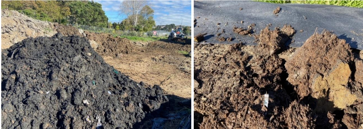
Figure 10. Portland Road, May 2022. Left: digger-excavated sediment shortly after deposition and before 'ageing', with gross contaminants visible and the stripped topsoil in the background. Right: flocculated geobag sediments showing the banding/layering that can occur over different excavation days: the surface layer is more fibrous than the underlying layer.
