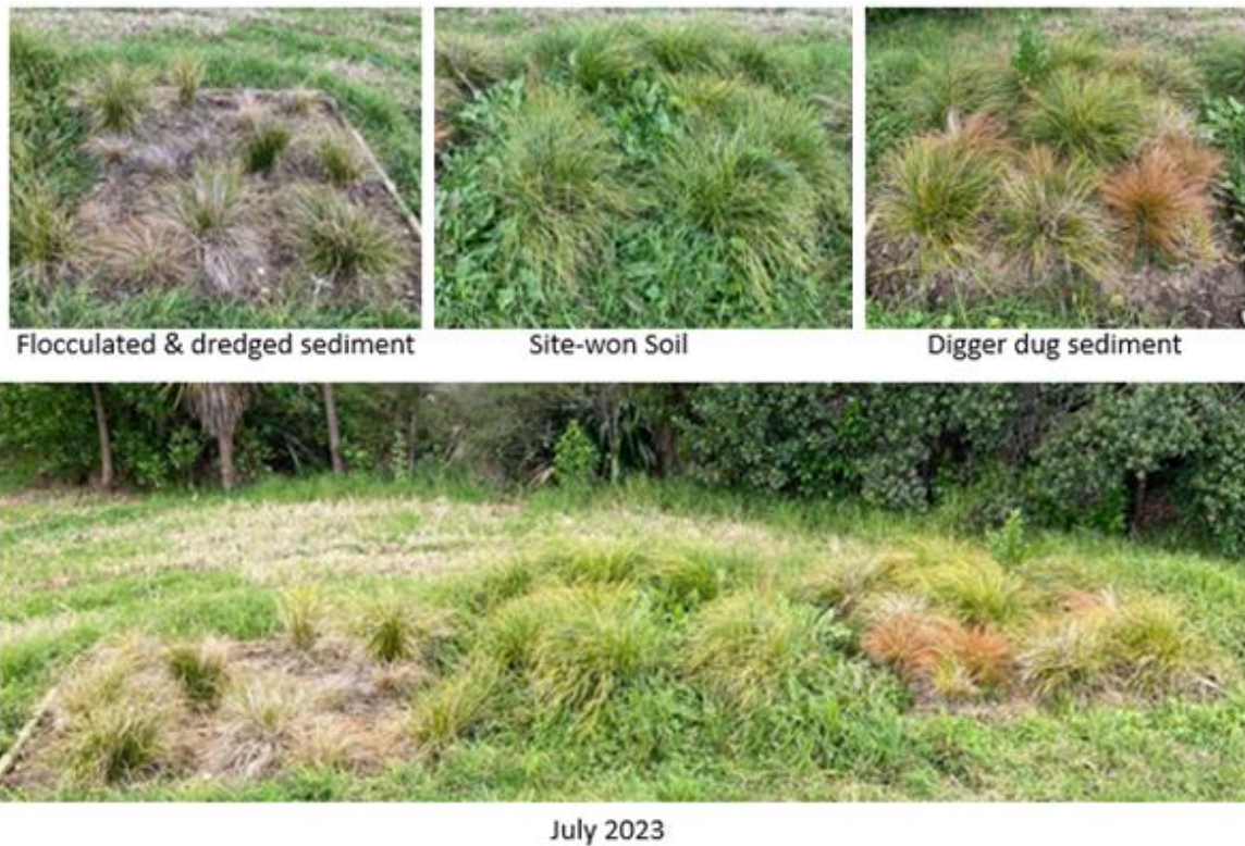
Figure 31. Portland Road trial, July 2023, showing taller sedges in the central topsoil plot and high cover of planted species in the digger-excavated sediment plot (right).
