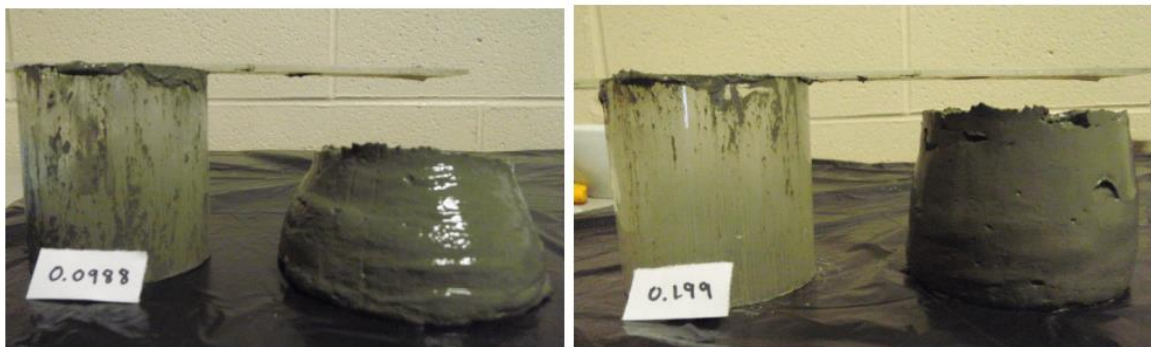
Figure 19. Examples of slump tests on sediment that has been consolidated. Source: TRCA 2018.
