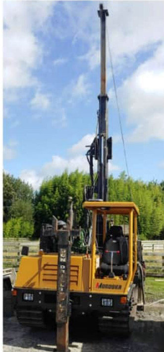
Figure 2-1: Photos of the Morooka drill rig and the instrumented SPT rod assembly.
