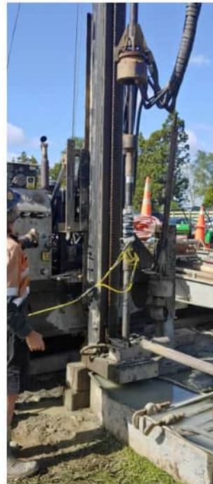
Figure 2-1: Photos of the Morooka drill rig and the instrumented SPT rod assembly.
