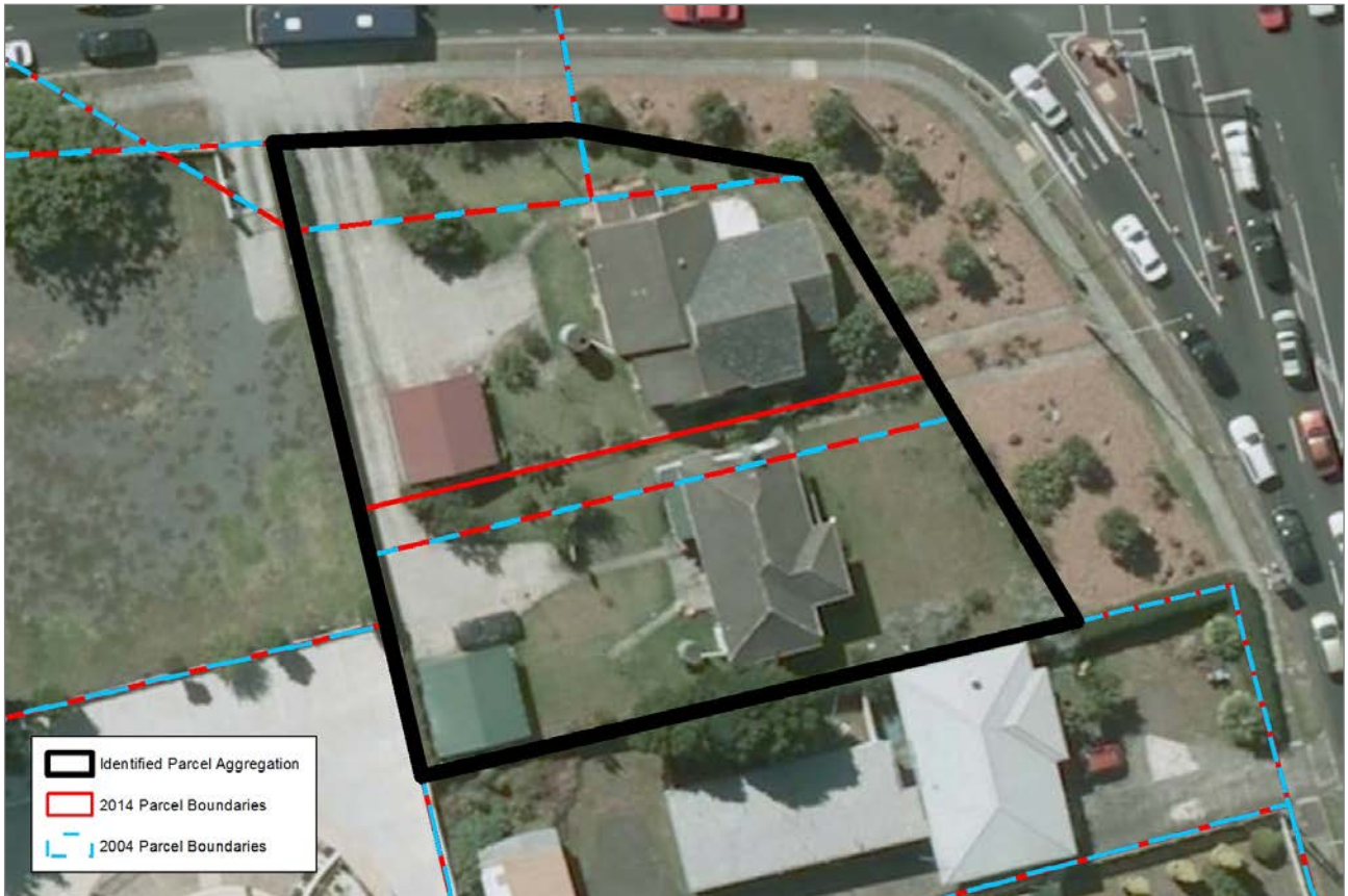
Figure 12: Example of creation of a new parcel in order to correct a boundary issue
