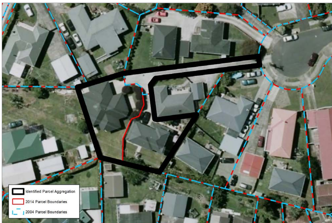
Figure 10: Example of basic subdivision of a single parcel, where a title has a part share in a vehicle access parcel.
