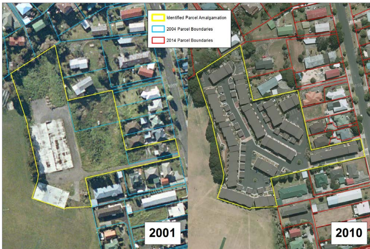
Figure 2: Example of property amalgamation (three parcels) resulting in the net loss of two parcels: development of site with higher-density residential
