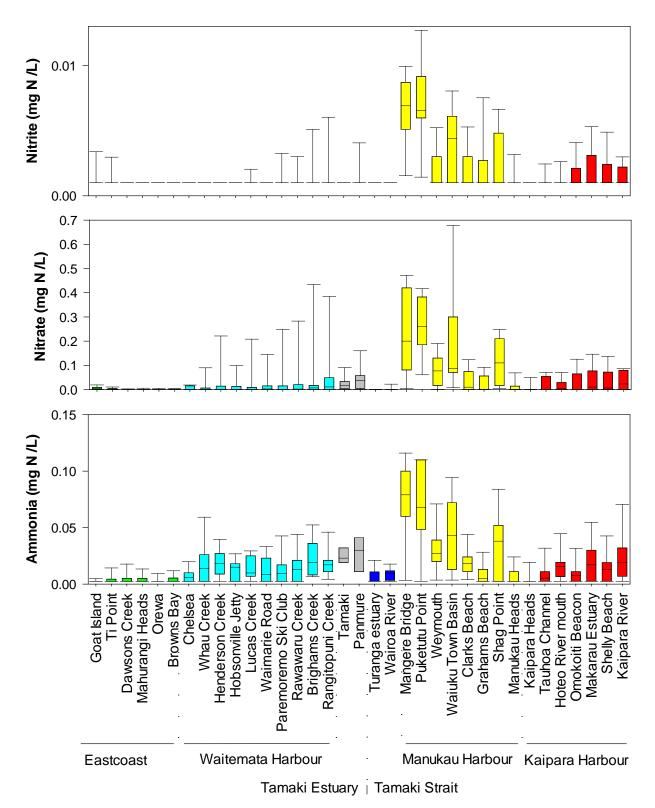
Figure 4-3 Spatial patterns in nitrite, nitrate and ammonia. Boxes represent the median, 25th and 75th percentiles while whiskers are 5th and 95th percentiles for data collected from January 2014 to December 2014. Percentiles values calculated using the standard method in SigmaPlot (v12).
