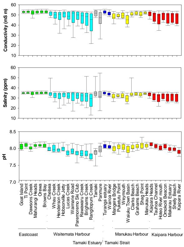
Figure 4-1 Spatial patterns in conductivity, salinity and pH. Boxes represent the median, 25th and 75th percentiles while whiskers are 5th and 95th percentiles for data collected from January 2014 to December 2014. Percentiles values calculated using the standard method in SigmaPlot (v12).
