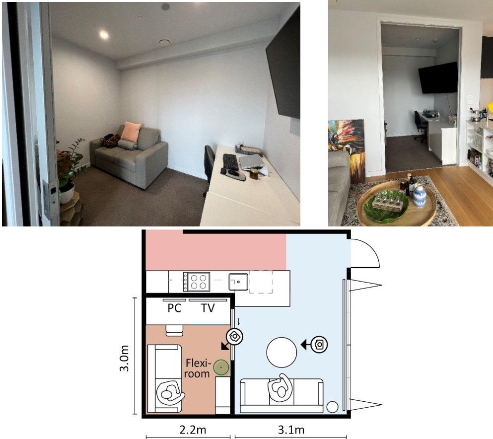
Figure 62: Flexi-room with glazed sliding door
