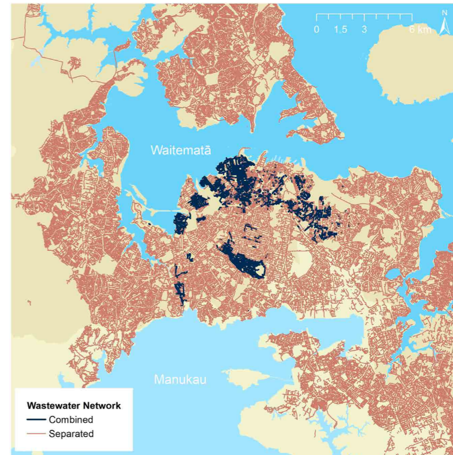
Figure 25: Central Auckland areas that have a combined wastewater and stormwater system, and areas that have a separated system.
