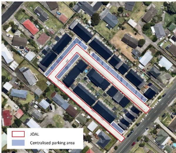
Figure 8: Example of a housing complex with a JOAL (Jointly Owned Access Lot), centralised parking, lighting, landscape treatment and pedestrian access
