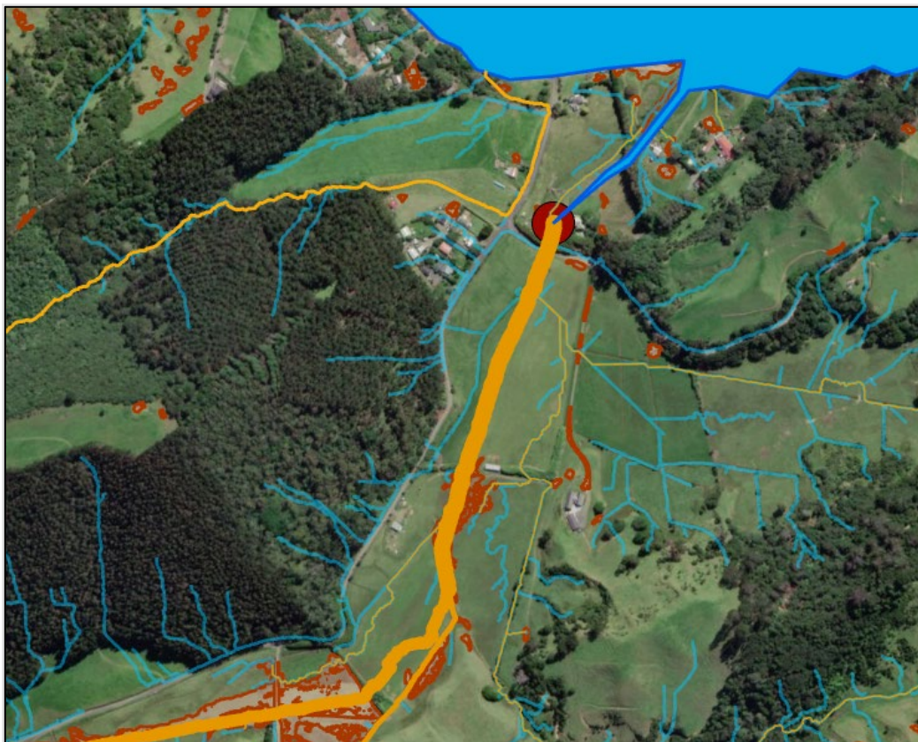
Figure 11: Example of relative predicted accumulation of sediment-like material post-Cyclone Gabrielle from bare earth areas (brown polygons) intersecting directly with overland flow paths (OLFPs; orange lines) to a potential coastal sink (brown circles) before entering the coastal marine environment (blue polygon).
