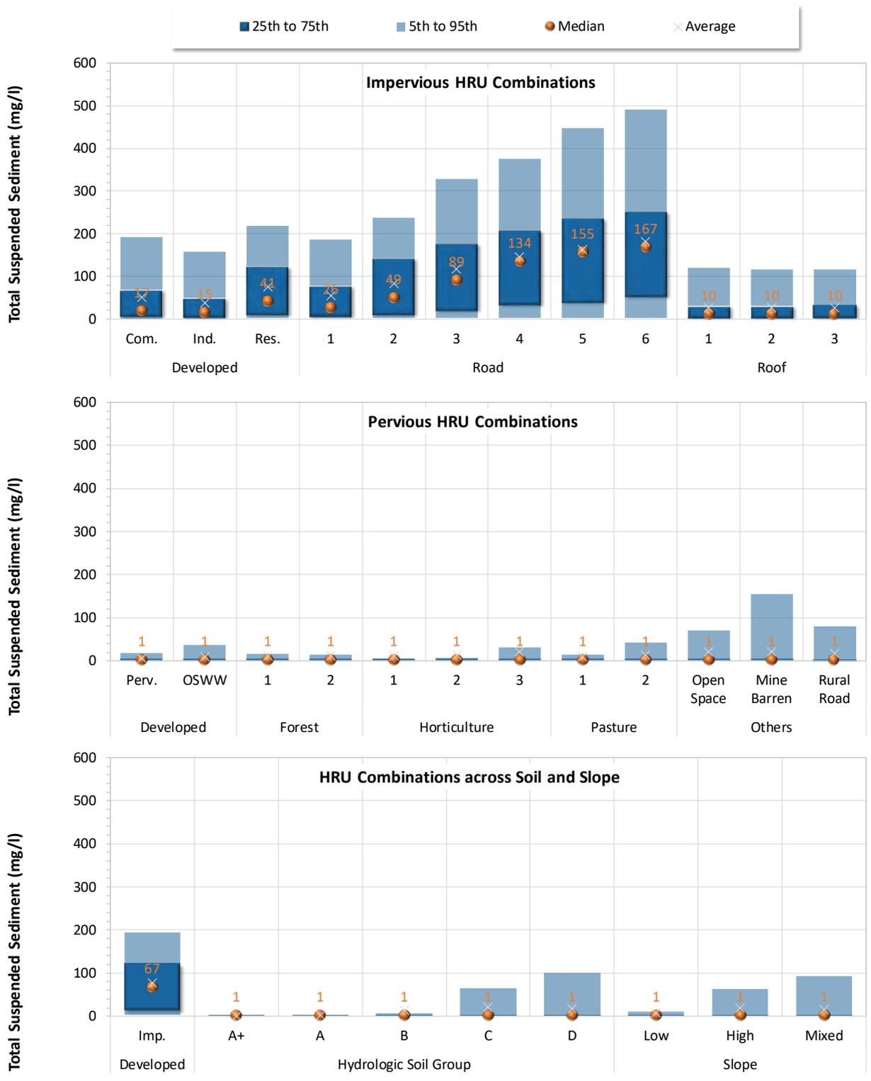
**Figure 4-50. HRU edge-of-stream daily average concentration (based on total water yield): Total Suspended Sediment (mg/l)**
