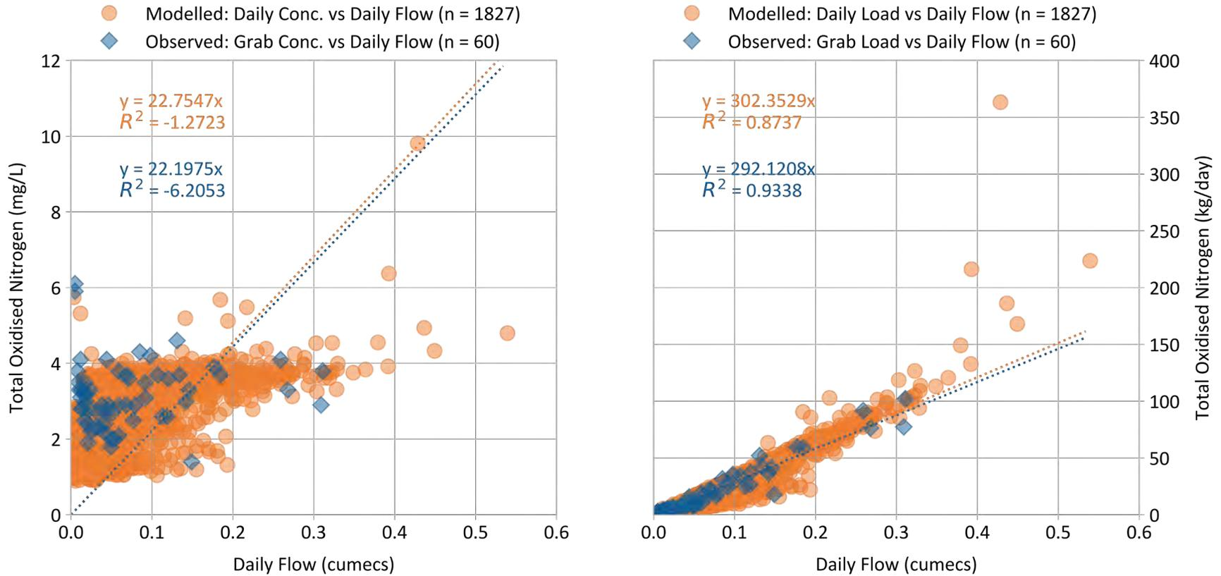
**Figure 4-45. Example Panel from Water Quality Calibration: Ngakoroa Stream @ Mill Rd (43829) – Total oxidised nitrogen calibration: Flow-based relationships for modelled daily (flow-weighted average) vs observed grab concentrations (left) and calculated grab sample loading rates (right) with linear scale. Note: the  $r^2$  values here are not relevant to calibration performance**
