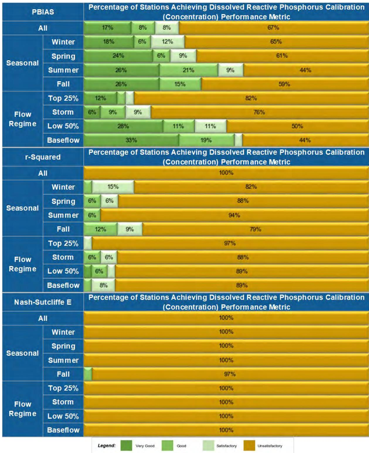
Figure 4-78. Dissolved reactive phosphorus (concentration) performance metrics for 36 Calibration and Validation AC SoE Stations
