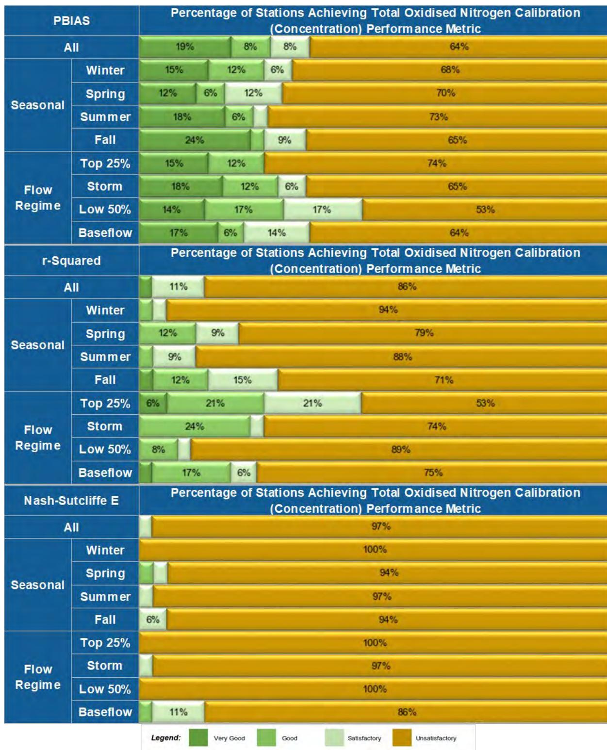
Figure 4-69. Total oxidised nitrogen (concentration) performance metrics for 36 Calibration and Validation AC SoE Stations
