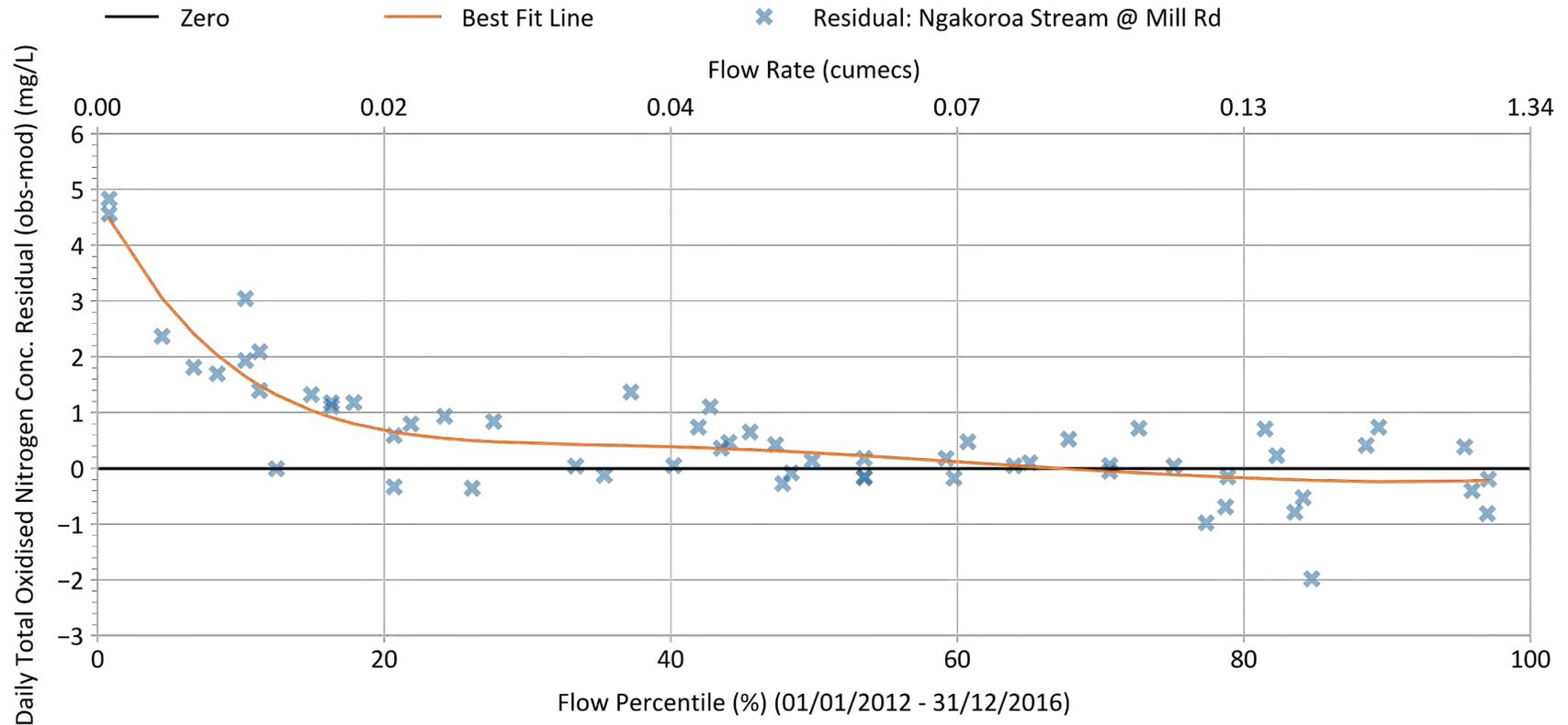
Figure 4-40. Example Panel from Water Quality Calibration: Ngakoroa Stream @ Mill Rd (43829) – Total oxidised nitrogen calibration: Modelled daily (flow-weighted average) vs observed grab sample concentration residual by observed daily average streamflow percentile
