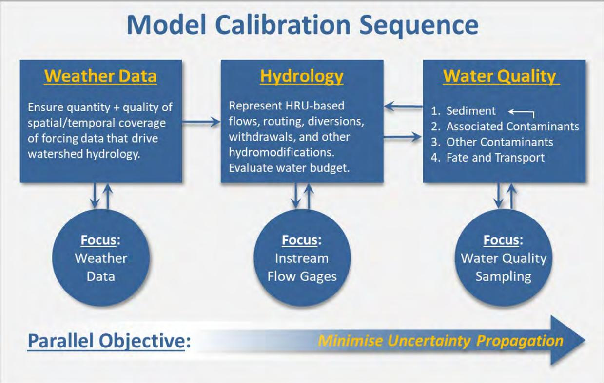
Figure 4-2. Top-down calibration sequence used for FWMT calibration
