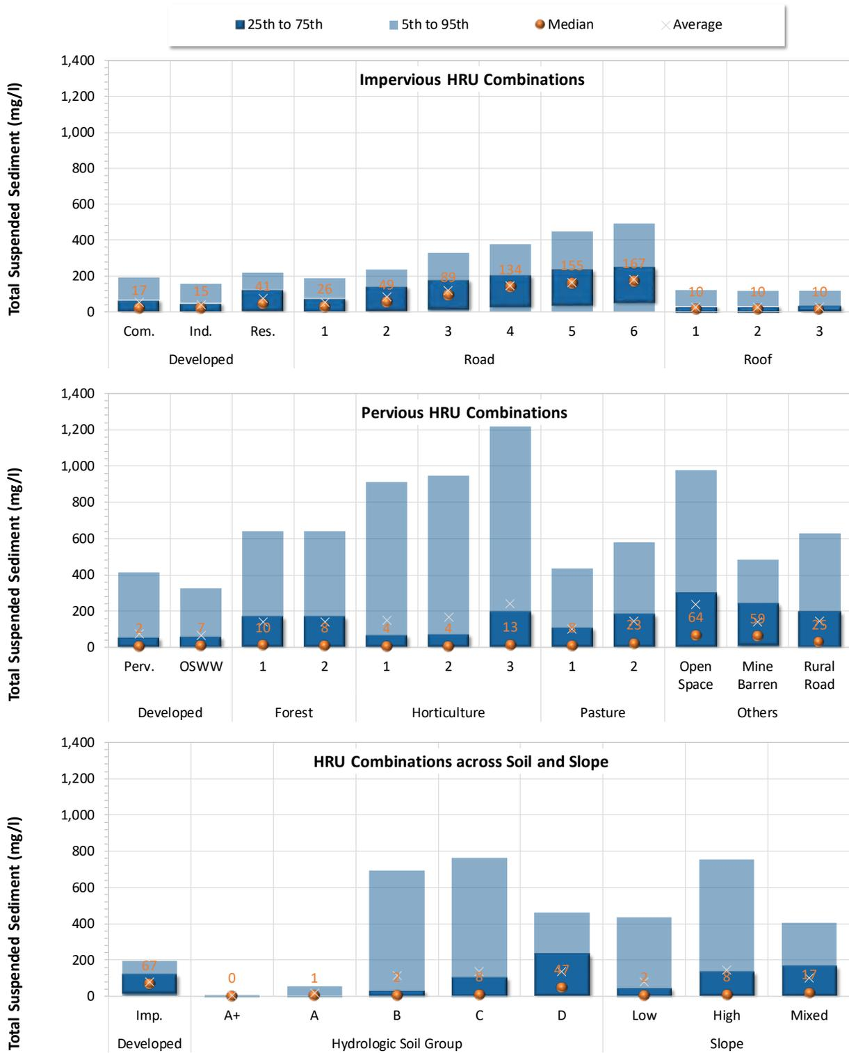
**Figure 4-49. HRU edge-of-stream daily average concentration (based on surface runoff): Total Suspended Sediment (mg/l)**
