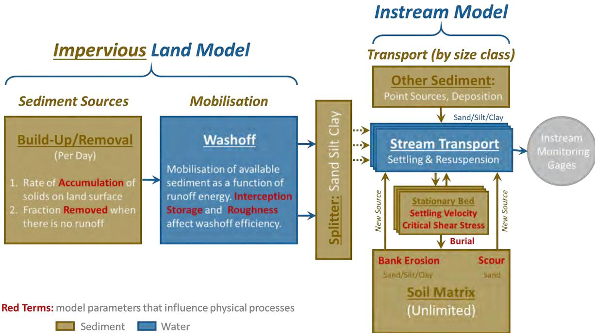
Figure 3-67. Sediment simulation process diagram for impervious surfaces upstream of instream transport
