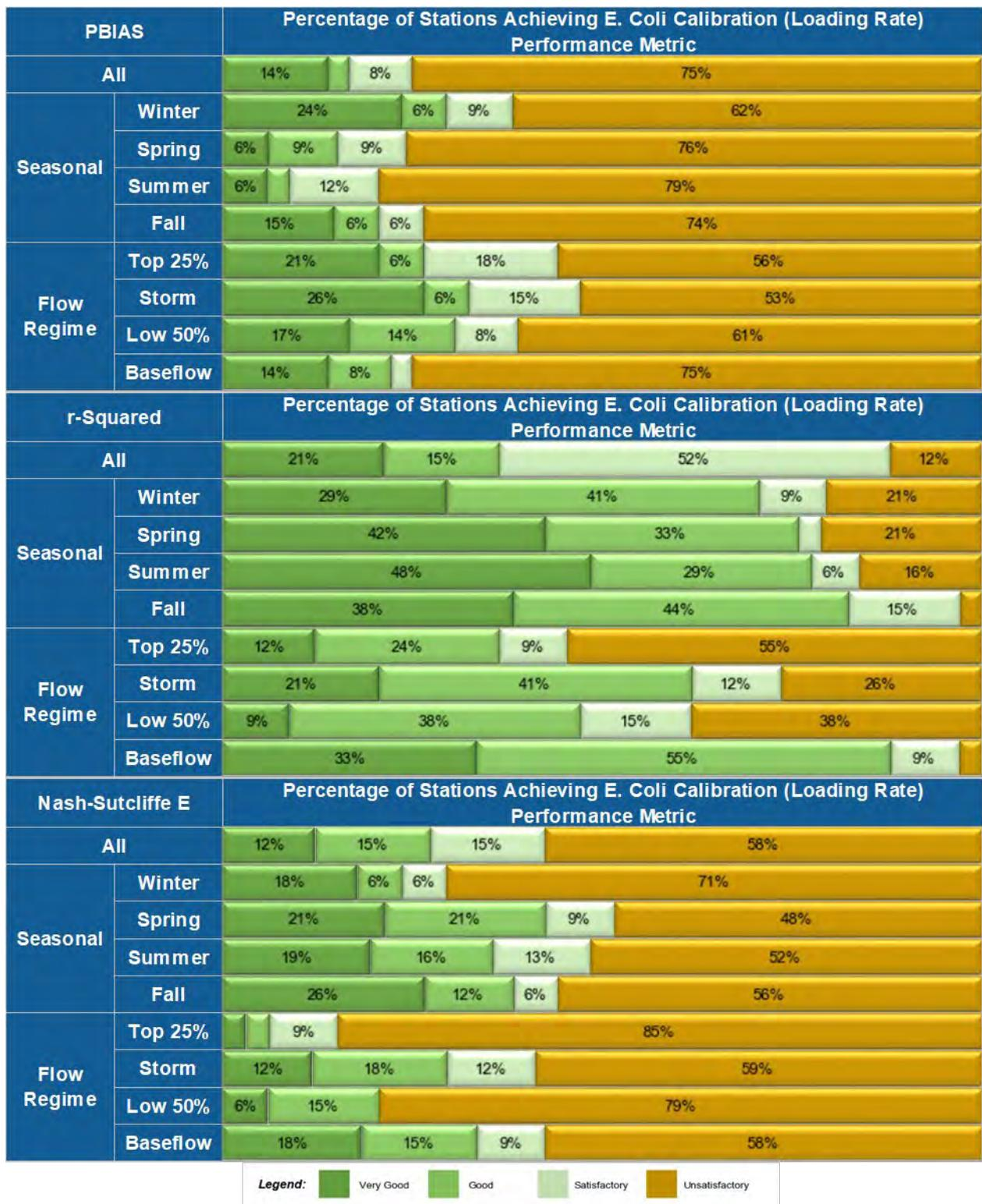
Figure 4-88. E. coli (load) performance metrics for 36 Calibration and Validation AC SoE Stations
