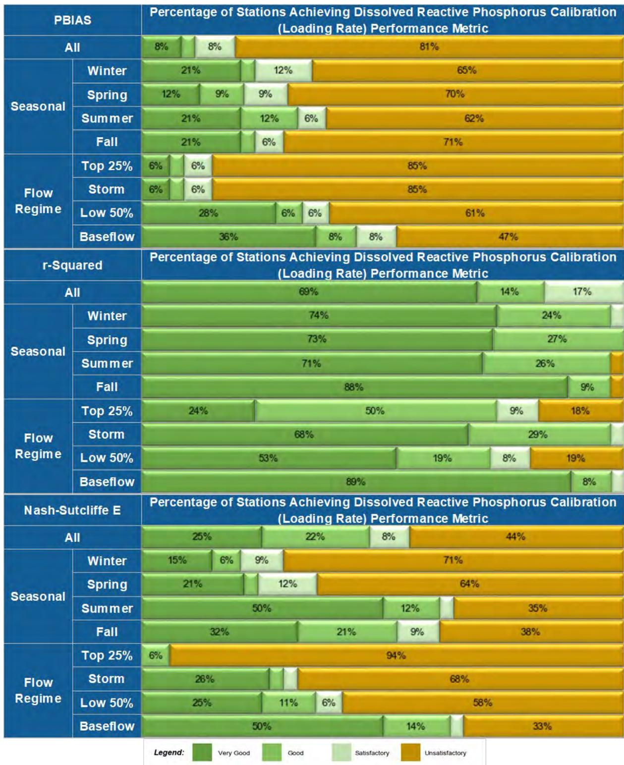
Figure 4-79. Dissolved reactive phosphorus (load) performance metrics for 36 Calibration and Validation AC SoE Stations
