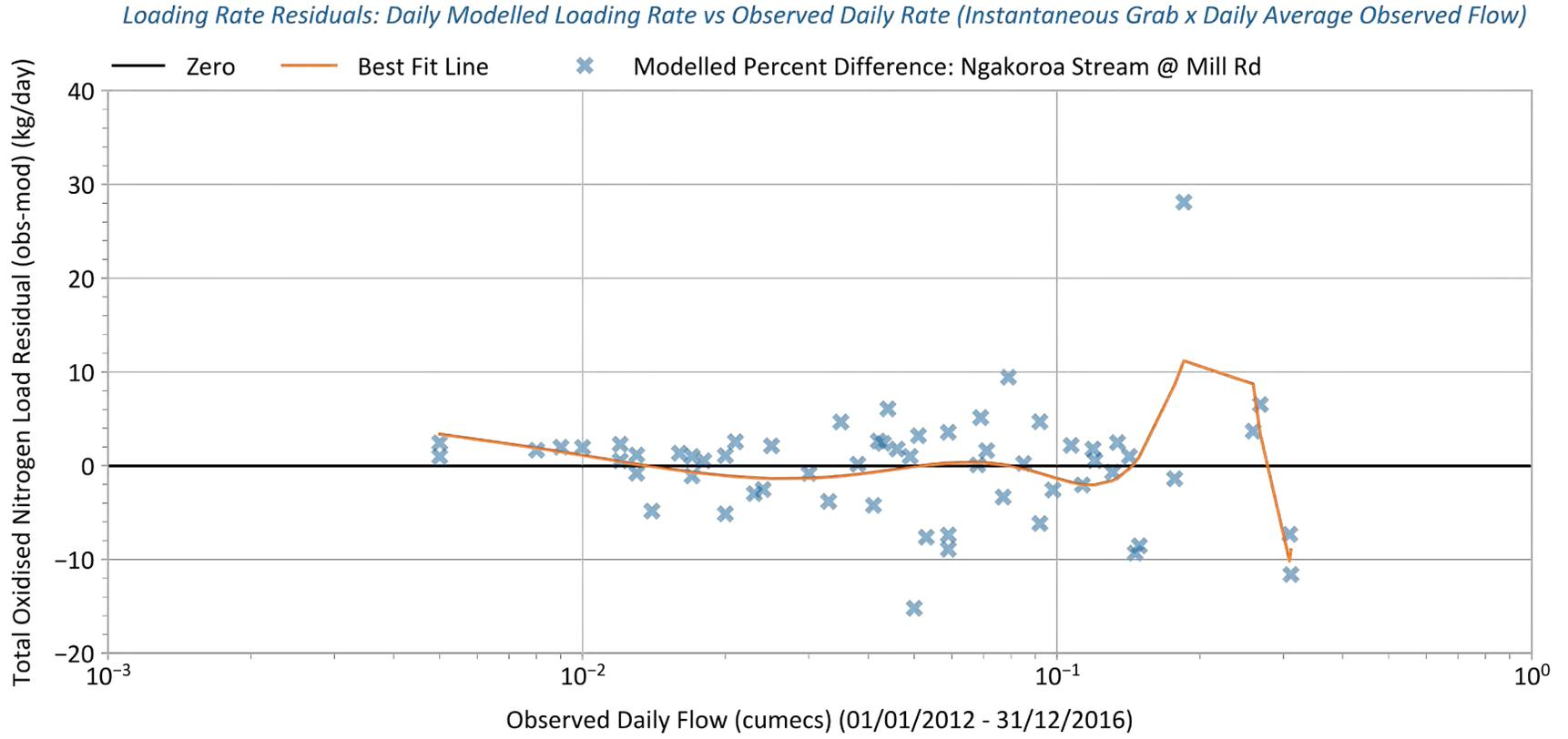
**Figure 4-42. Example Panel from Water Quality Calibration: Ngakoroa Stream @ Mill Rd (43829) – Total oxidised nitrogen calibration: Modelled daily (flow-weighted average) vs calculated grab sample loading rate residual by observed daily average streamflow on sampling dates**
