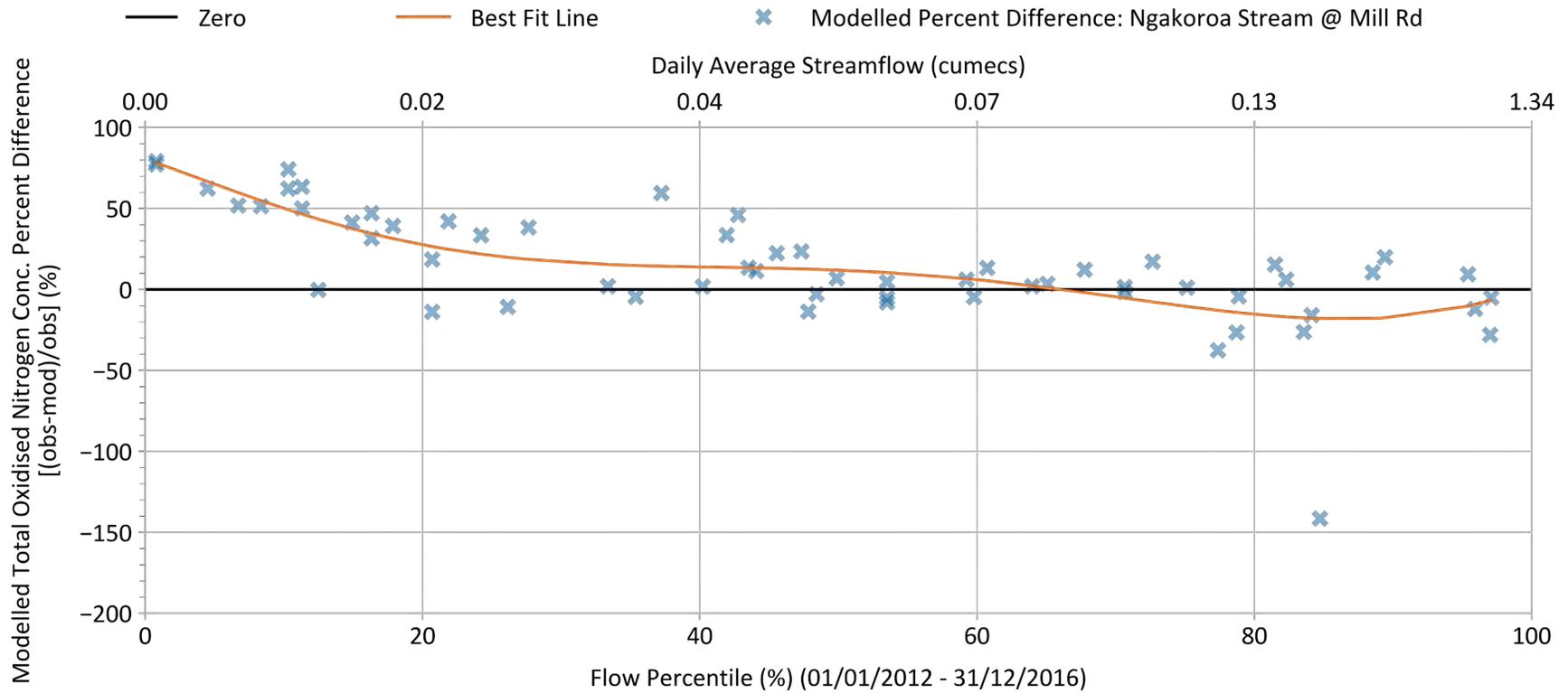
**Figure 4-39. Example Panel from Water Quality Calibration: Ngakoroa Stream @ Mill Rd (43829) – Total oxidised nitrogen calibration: Modelled daily (flow-weighted average) vs observed grab sample concentration per cent difference by observed daily average streamflow percentile**
