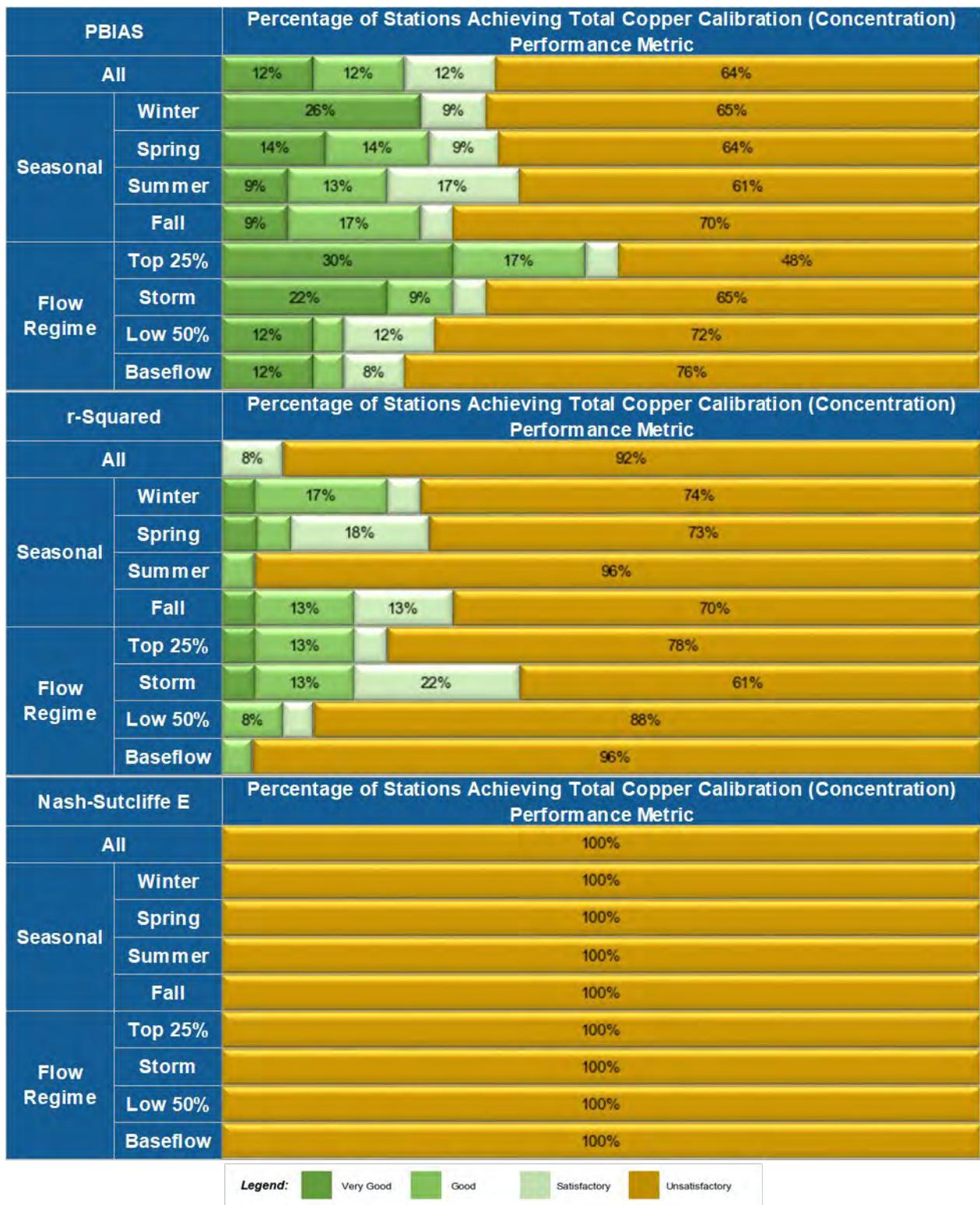
Figure 4-81. Total copper (concentration) Performance at 25 Calibration and Validation AC SoE Stations
