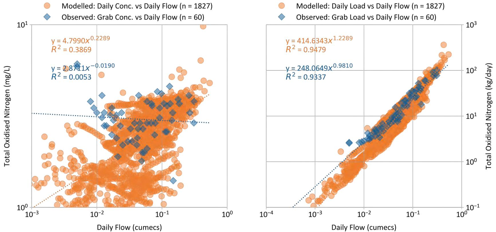
**Figure 4-46. Example Panel from Water Quality Calibration: Ngakoroa Stream @ Mill Rd (43829) – Total oxidised nitrogen calibration: Flow-based relationships for modelled daily vs observed grab concentrations (left) and calculated grab sample loading rates (right) with log scale. Note: R<sup>2</sup> values here are not relevant to calibration performance**
