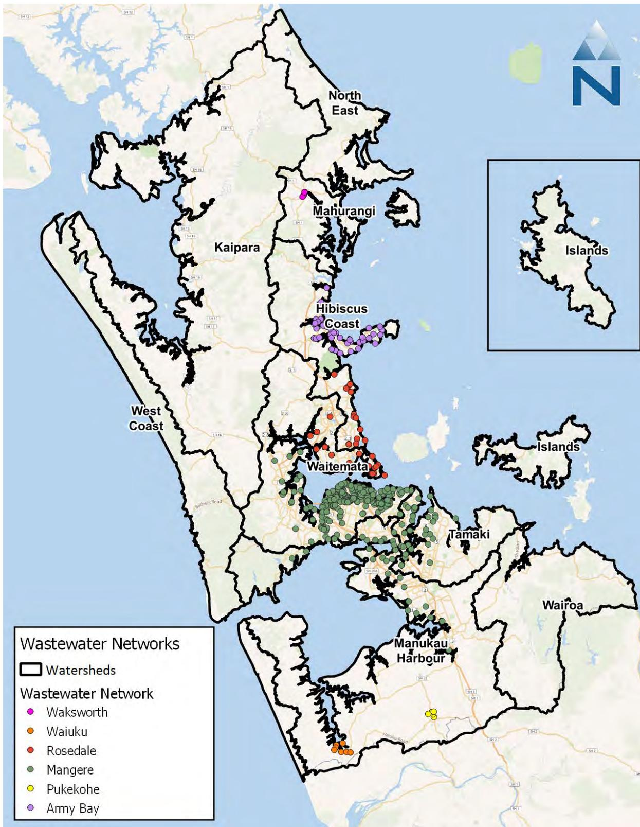
**Figure 3-9. Wastewater conveyance network service areas and all engineered overflow points (EOPs) represented in the FWMT Stage 1**
