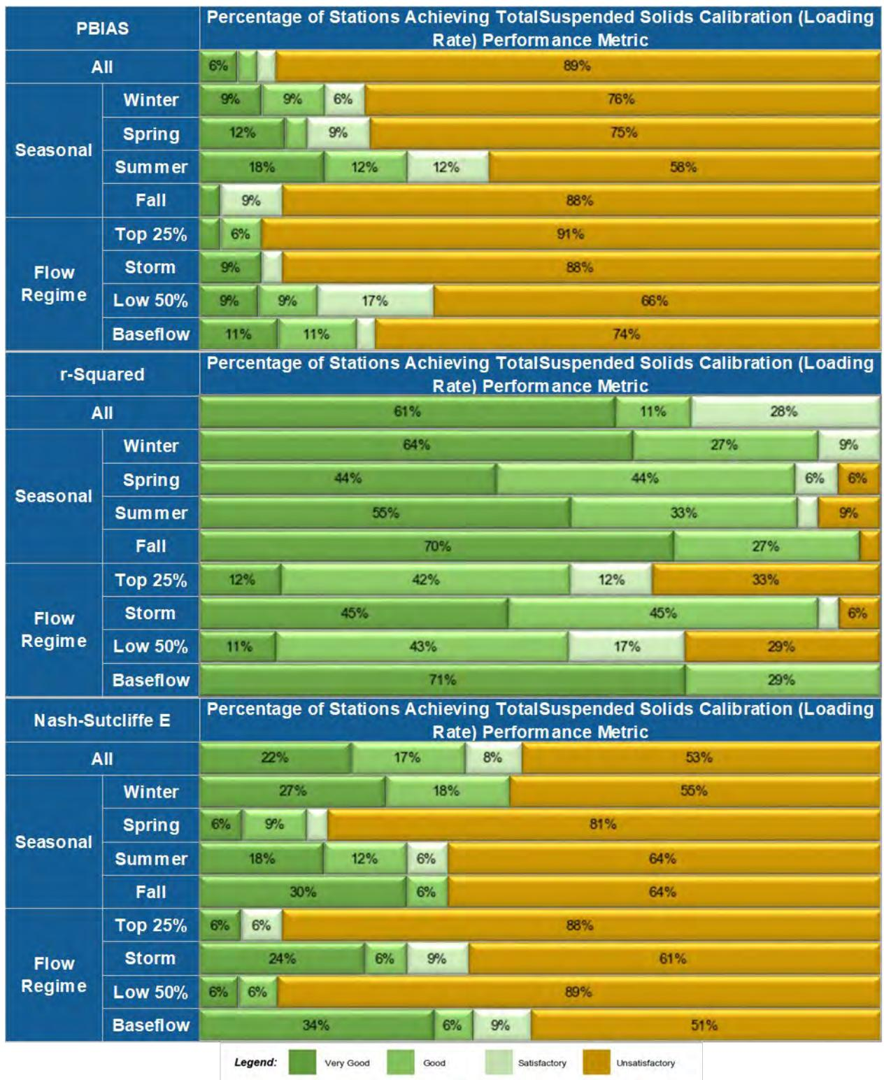
Figure 4-64. Total suspended solids (load) performance metrics for 36 Calibration and Validation SoE Stations (including 10 stations with co-located flow records)
