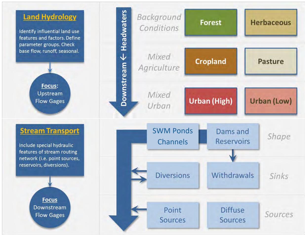
**Figure 4-3. Upstream-downstream sequence used for FWMT calibration**
