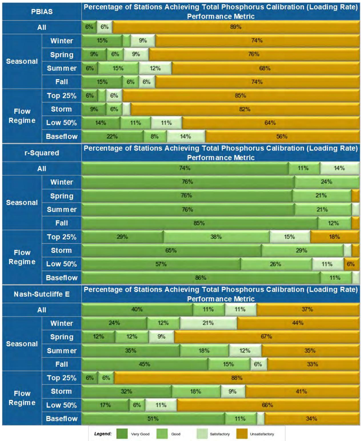
Figure 4-76. Total phosphorus (load) performance metrics for 36 Calibration and Validation AC SoE Stations
