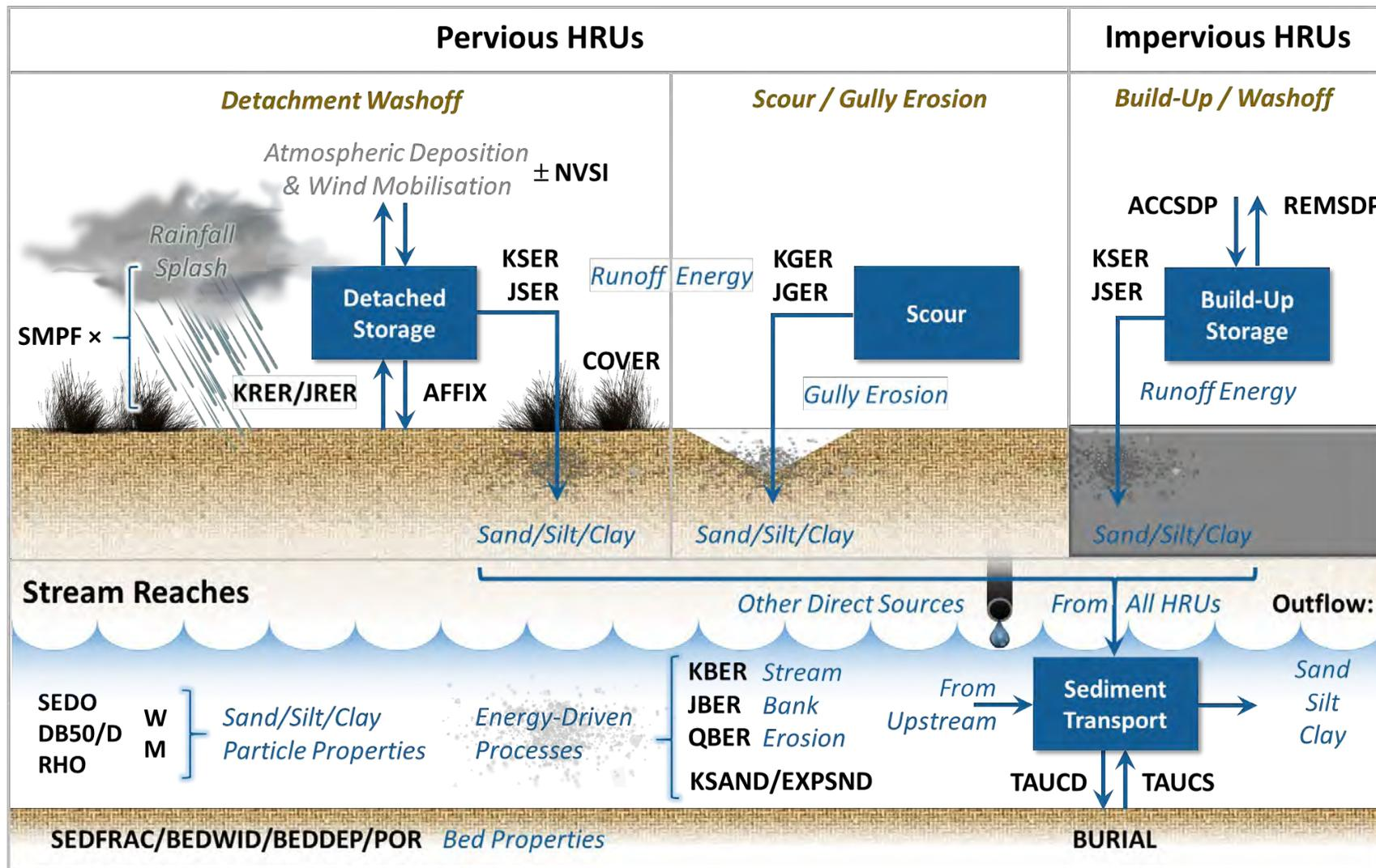
Figure 2-7. Schematic of sediment routines and parameters in LSPC
