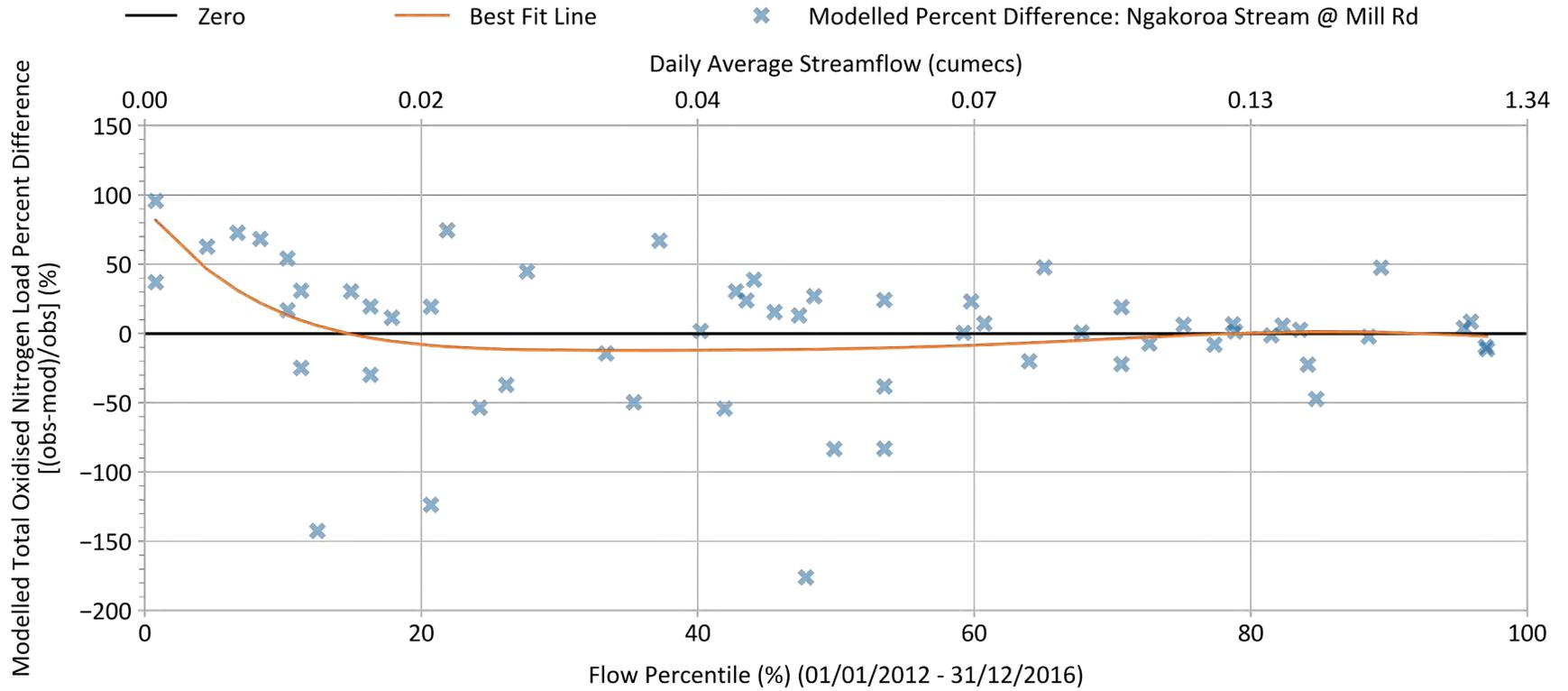
**Figure 4-43. Example Panel from Water Quality Calibration: Ngakoroa Stream @ Mill Rd (43829) – Total oxidised nitrogen calibration: Modelled daily (flow-weighted average) vs calculated grab sample loading rate per cent difference by observed daily average streamflow percentile**
