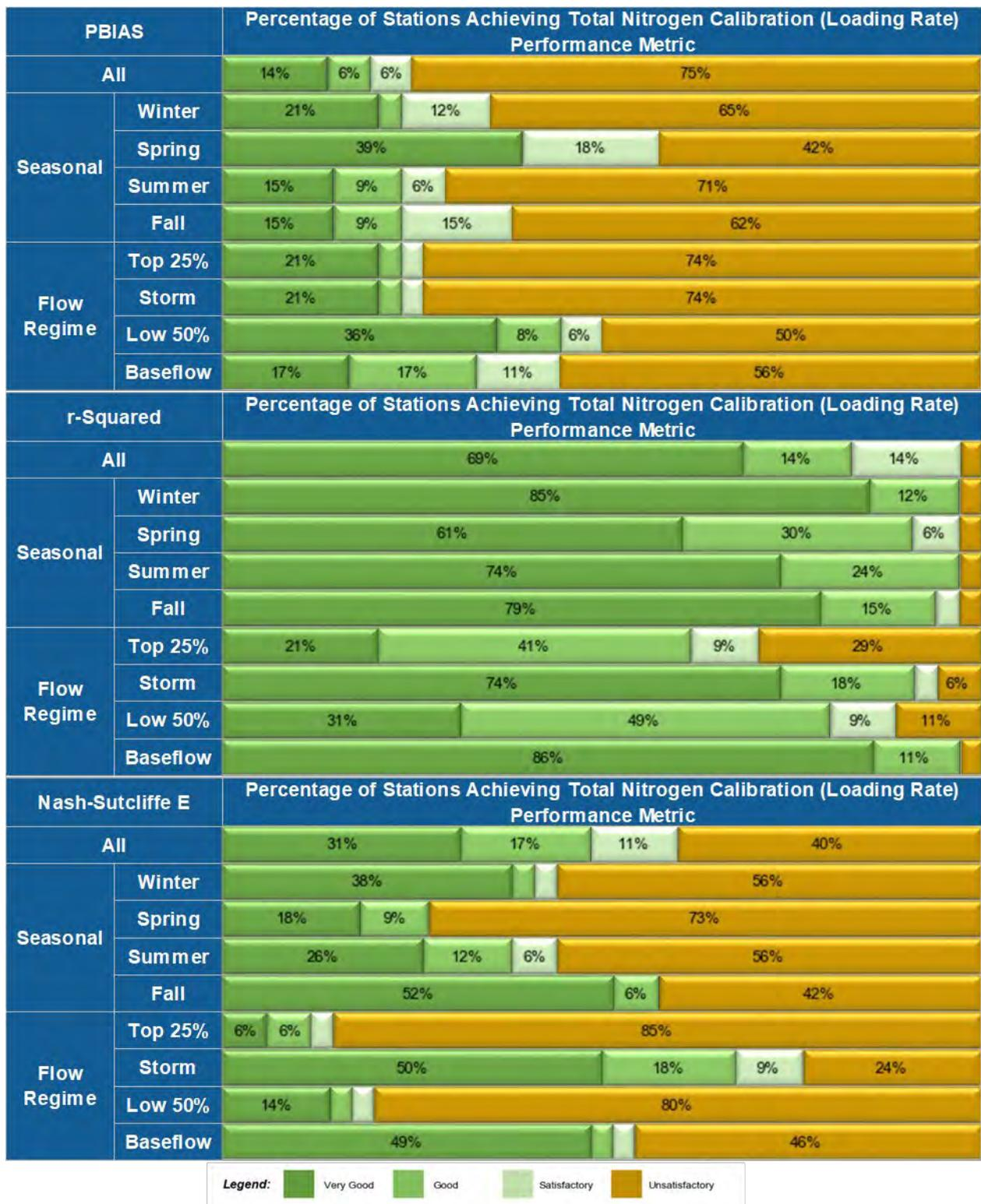
Figure 4-67. Total nitrogen (load) performance metrics for 36 Calibration and Validation AC SoE Stations
