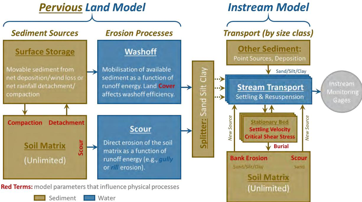
**Figure 3-68. Sediment simulation process diagram for pervious surfaces upstream of instream transport**
