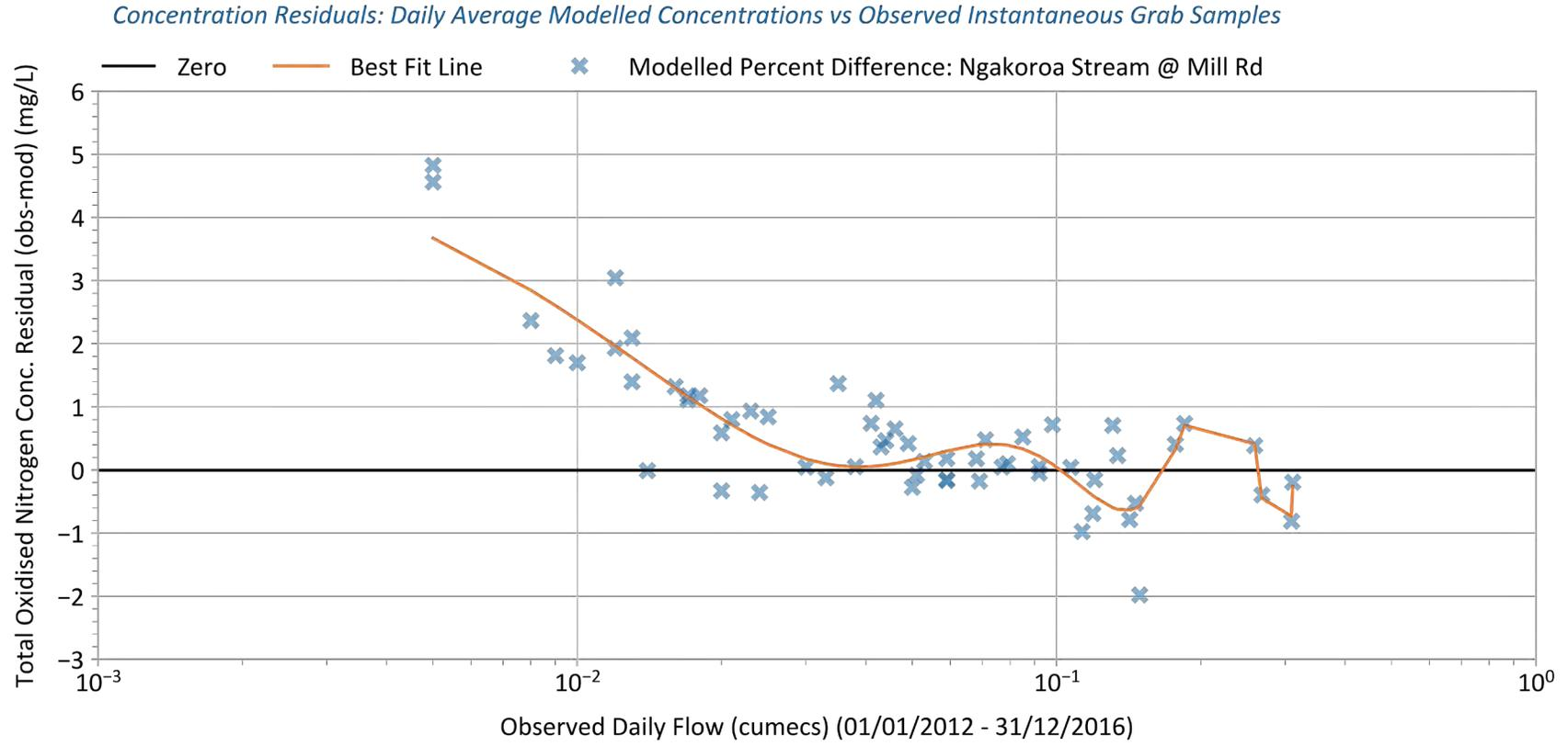
**Figure 4-38. Example Panel from Water Quality Calibration: Ngakoroa Stream @ Mill Rd (43829) – Total oxidised nitrogen calibration: Modelled daily (flow-weighted average) vs observed grab sample concentration residual by observed daily average streamflow on sampling dates**
