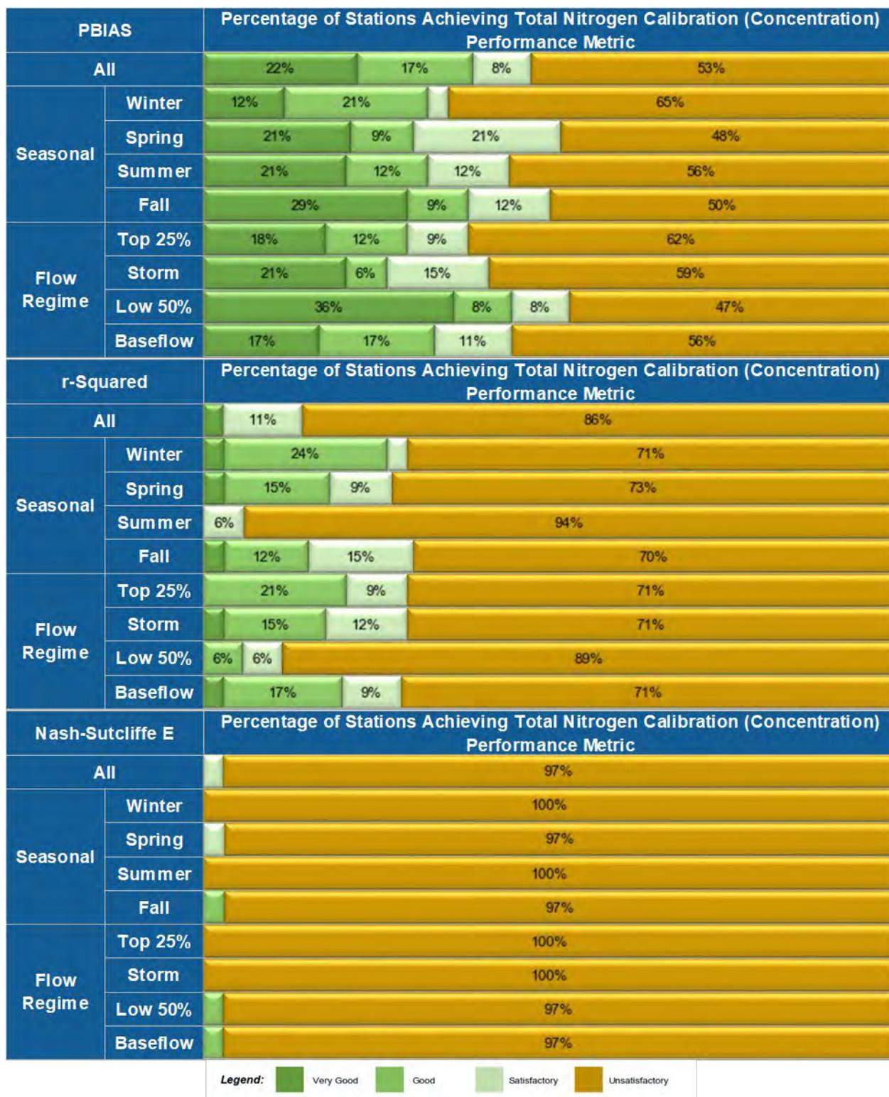
Figure 4-66. Total nitrogen (concentration) Performance Metrics for Calibration and Validation AC SoE Stations
