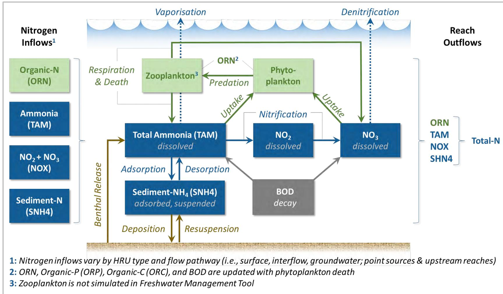
Figure 2-8. Schematic of nitrogen / RQUAL routines and parameters in LSPC<sup>3</sup>
