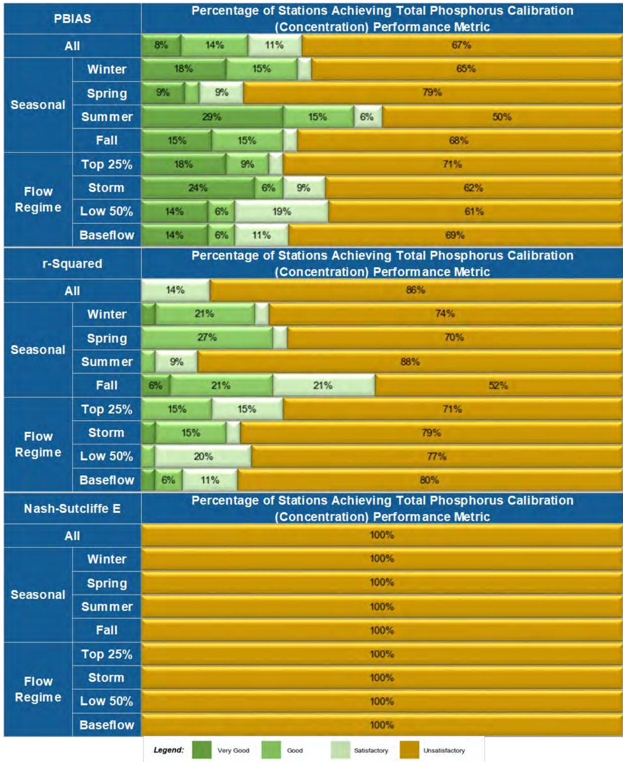
Figure 4-75. Total phosphorus (concentration) performance metrics for 36 Calibration and Validation AC SoE Stations
