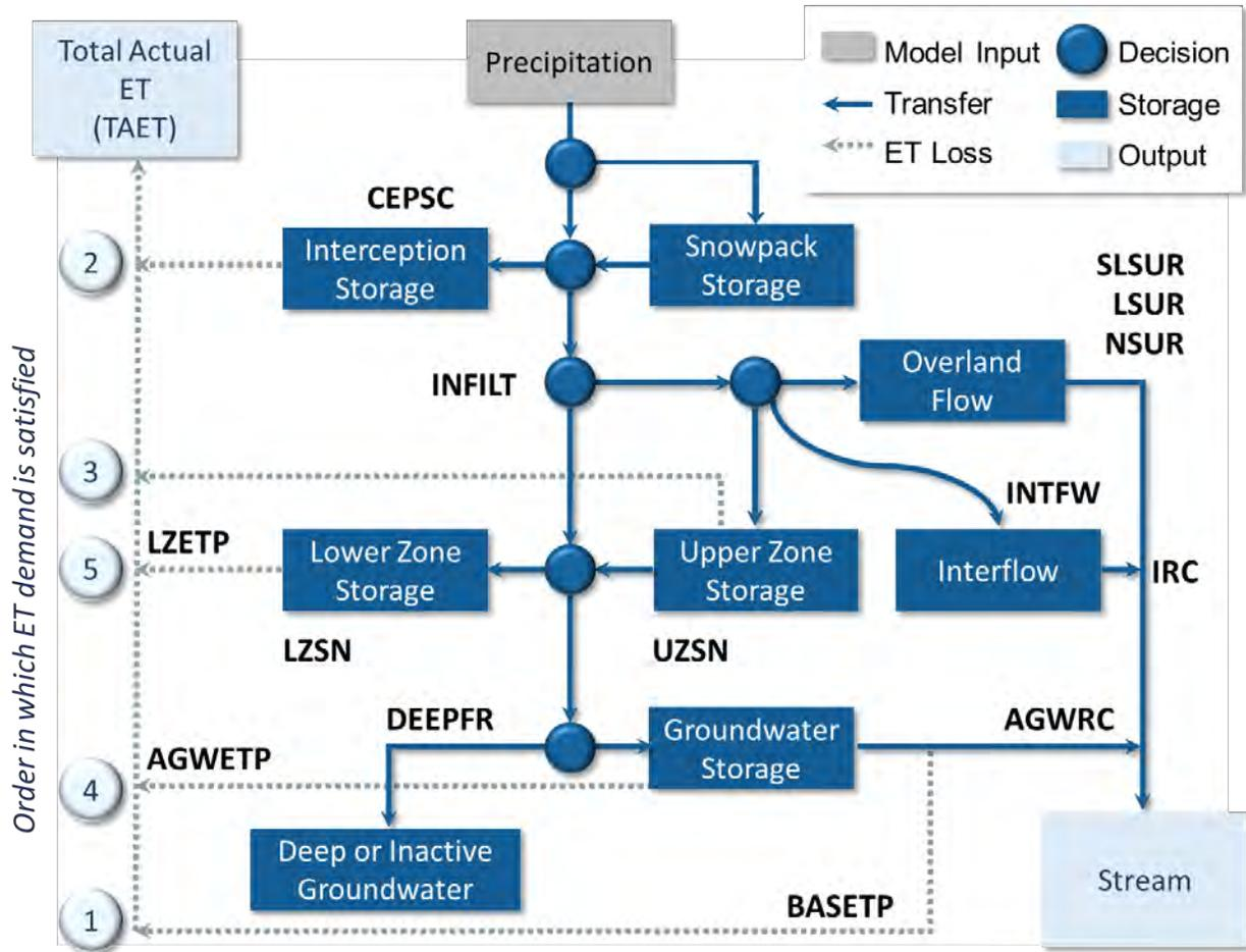
Figure 2-6. Schematic of hydrology component and routines/parameters in LSPC
