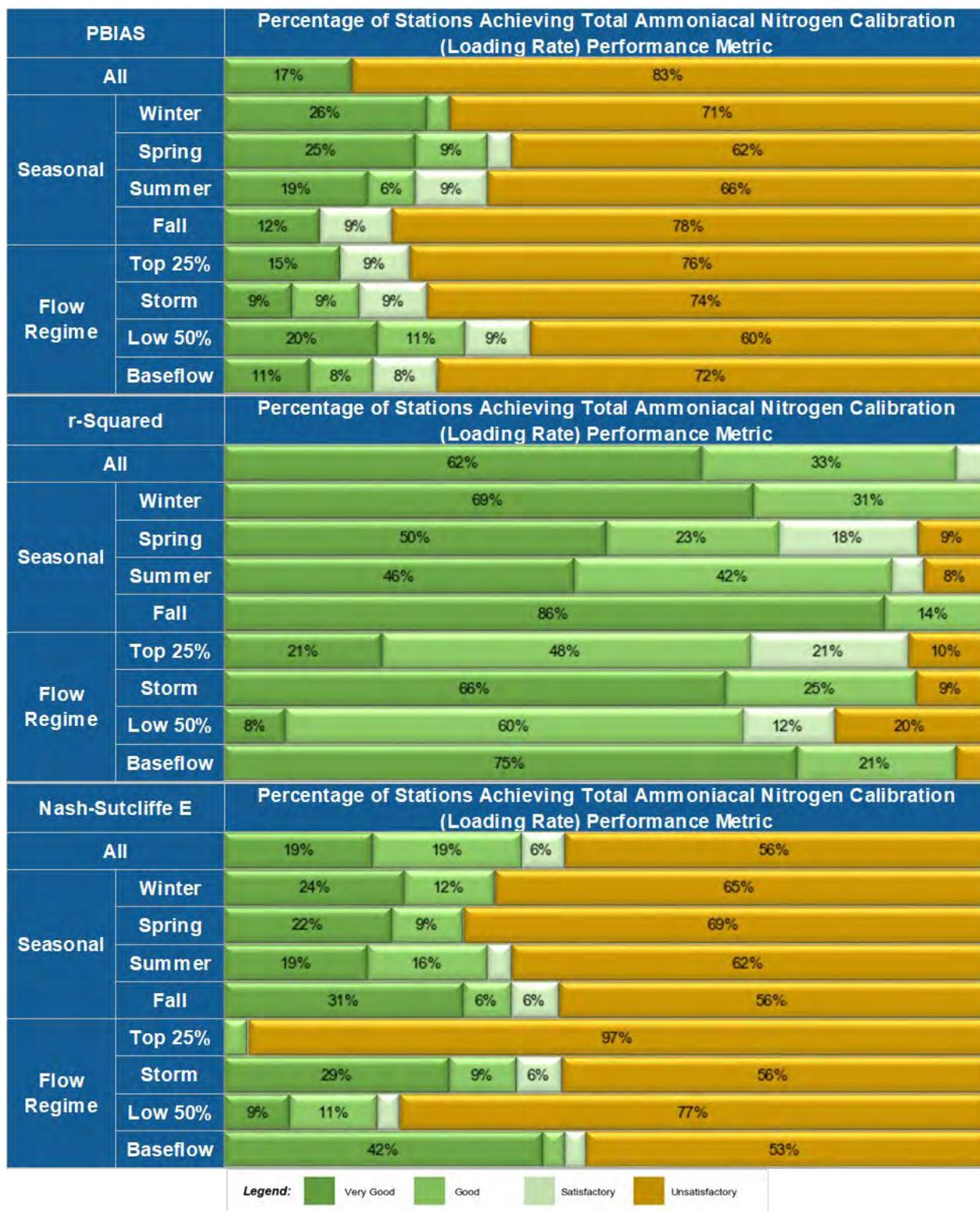
**Figure 4-73. Total ammoniacal nitrogen (load) performance metrics for 36 Calibration and Validation AC SoE Stations**
