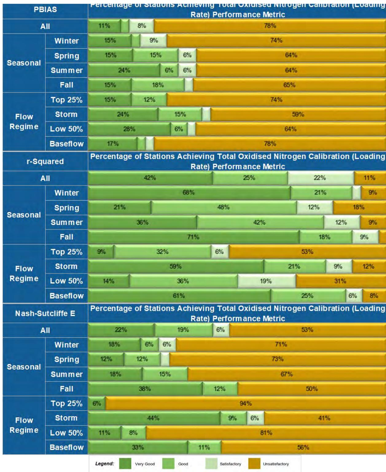
Figure 4-70. Total oxidised nitrogen (load) performance metrics for 36 Calibration and Validation AC SoE Stations
