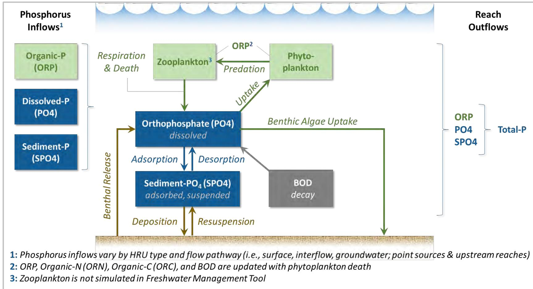
**Figure 2-9. Schematic of phosphorus / RQUAL routines and parameters in LSPC**
