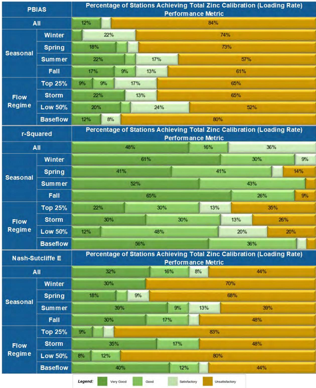
Figure 4-85. Total zinc (load) Performance at 25 Calibration and Validation AC SoE Stations
