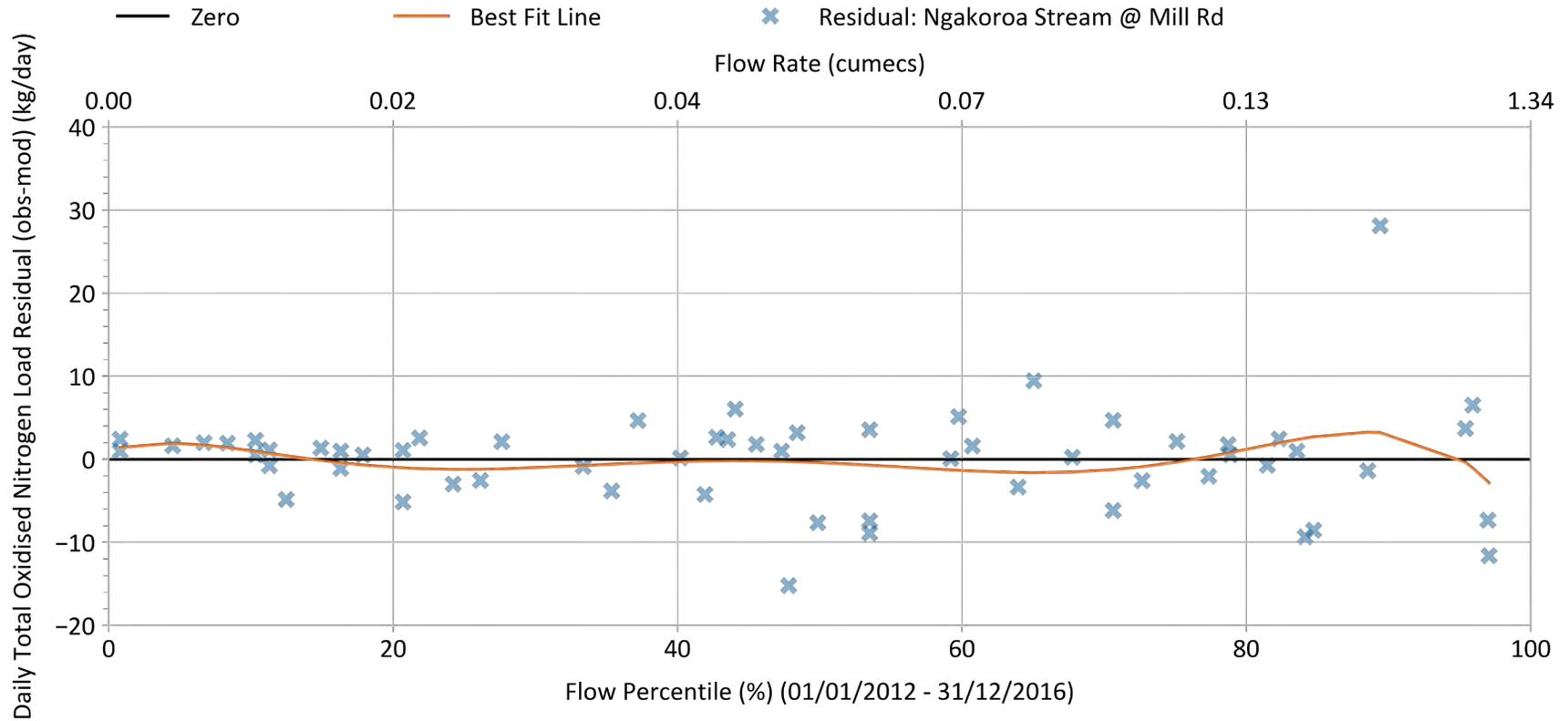
Figure 4-44. Example Panel from Water Quality Calibration: Ngakoroa Stream @ Mill Rd (43829) – Total oxidised nitrogen calibration: Modelled daily (flow-weighted average) vs calculated grab sample loading rate residual by observed daily average streamflow percentile
