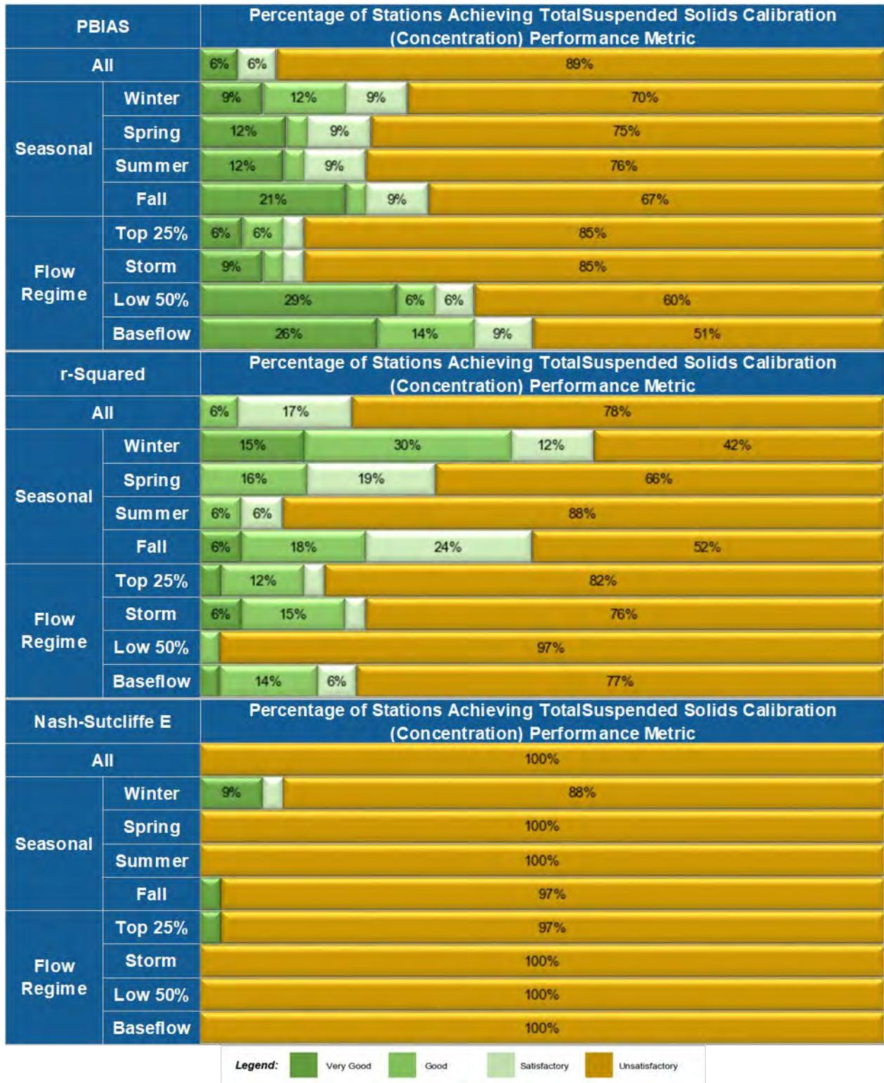
Figure 4-63. Total suspended solids (concentration) performance metrics for 36 Calibration and Validation SoE Stations (including 10 stations with co-located flow records)
