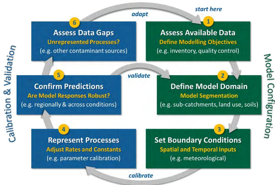
Figure 2-4. Conceptual schematic of a LSPC model development cycle for the FWMT
