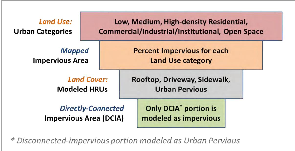
Figure 3-60. Translation Sequence from Mapped Impervious Area to Directly Connected Impervious Area
