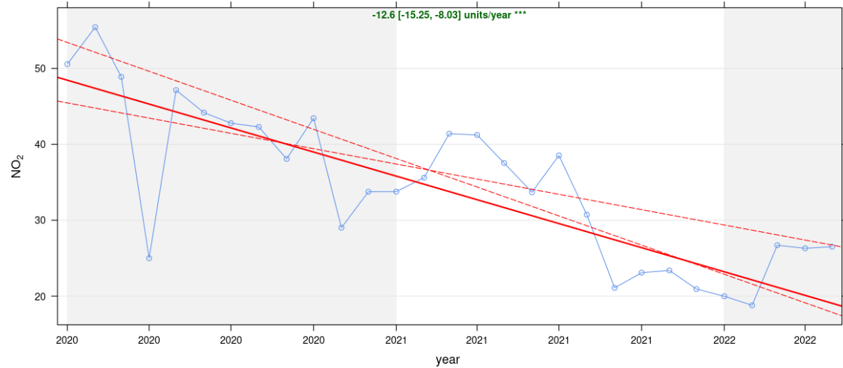
Figure 11. Trends in NO 2 at Customs Street. The plot shows the deseasonalised monthly mean concentrations of NO 2 . The solid red line shows the trend estimate and the dashed red lines show the 95% confidence intervals for the trend based on resampling methods. The overall trend is shown at the top-left as - 12.6 (µg/m 3 ) per year and the 95% confidence intervals in the slope from -15.25 – (- 8.03) µg/m 3 /year. The ‘***’ show that the trend is significant to the 0.001 level.
