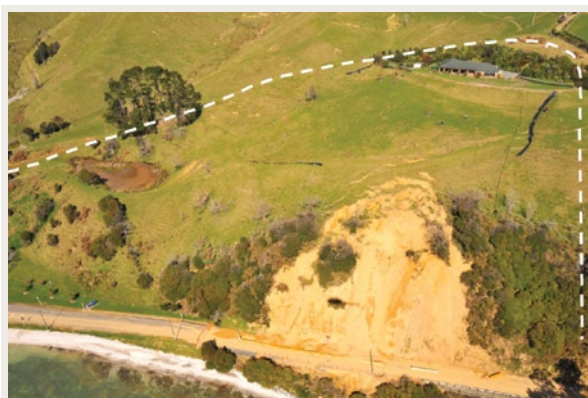
FIGURE 1 Aerial view of the 24 August 2008 landslide that blocked the Clevedon-Kawakawa Bay Road. The larger landslide which threatened a house is indicated by the white dash line. (Source: Manukau City Council).
