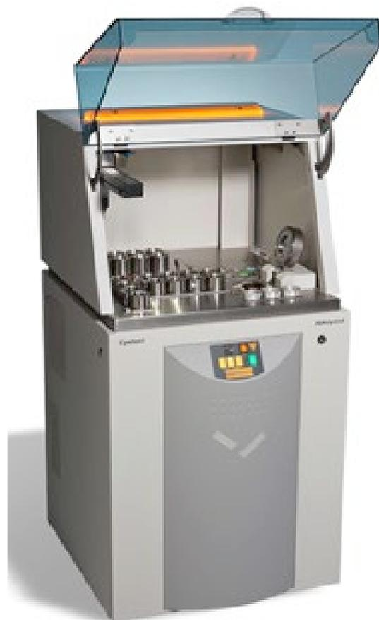
Figure A1.5 The PANalytical Epsilon 5 spectrometer.
