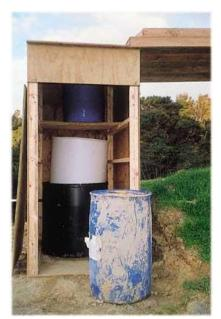
Figure 99: Rainfall activated flocculant treatment device
