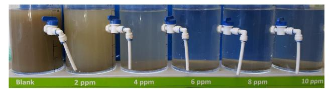
Figure 137: Example of test results from bench testing
