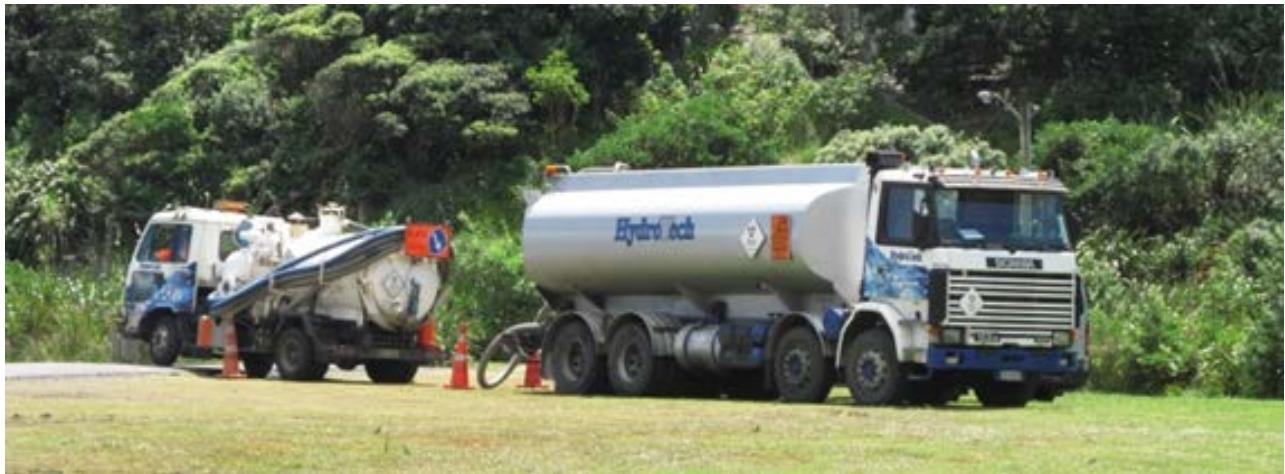
Septic tank pump out truck at Piha Domain 2017.
