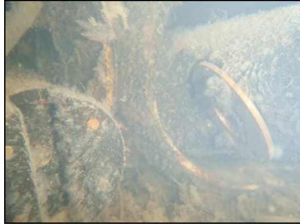
Figure 4: Sensors at Meo_MID_AAG site have experienced rapid algal growth reducing accuracy of the equipment.
