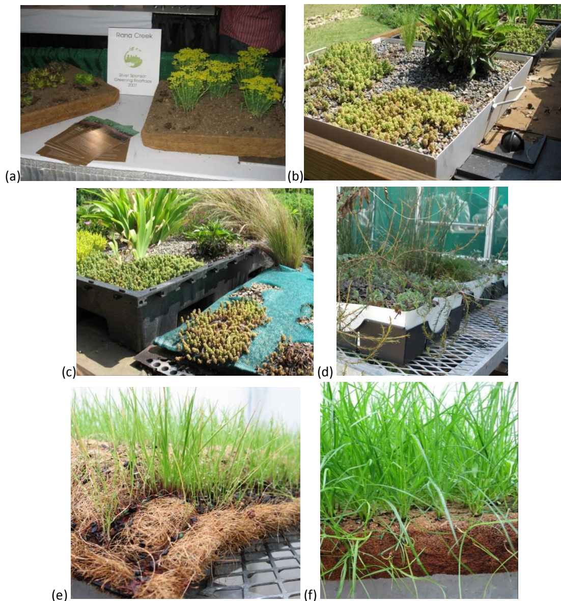
Figure 5. Ready-to-install modular systems; (a) coir trays (USA); (b) Aluminium and plastic 100 mm modular trays (USA); (c) 220 mm plastic tray and 100 mm modular bag (USA); (d) plastic 100 mm modular system with removable divider panels (NZ) (e) flexible coir pouch and (f) rigid coir pouch systems (NZ, imported).
