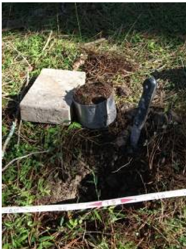
Figure 2. An intact soil core used to establish the physical quality of the soil.
