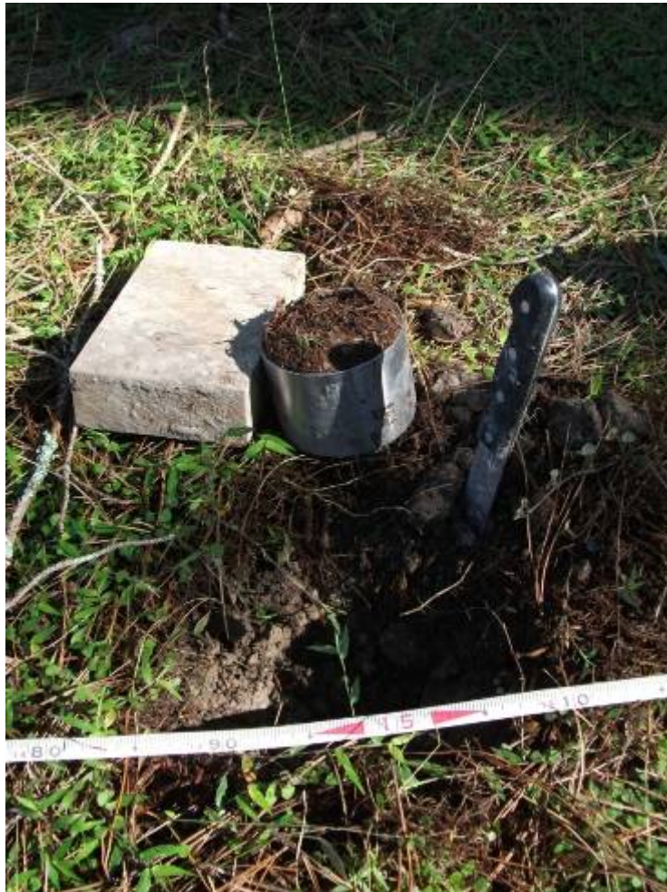
Figure 2. An intact soil core used to establish the soil physical quality of the soil.
