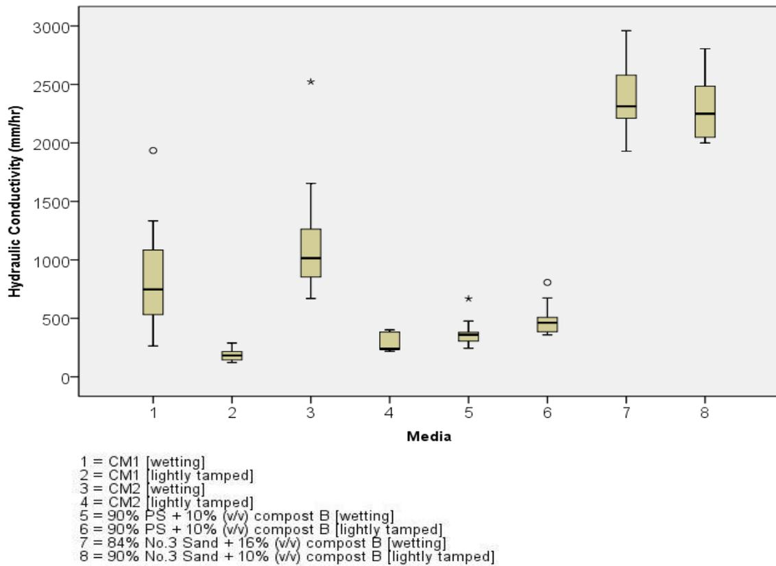
Figure 19 Effect of aggregate type on saturated hydraulic conductivity of bioretention filter media mixes (all compacted by wetting)
