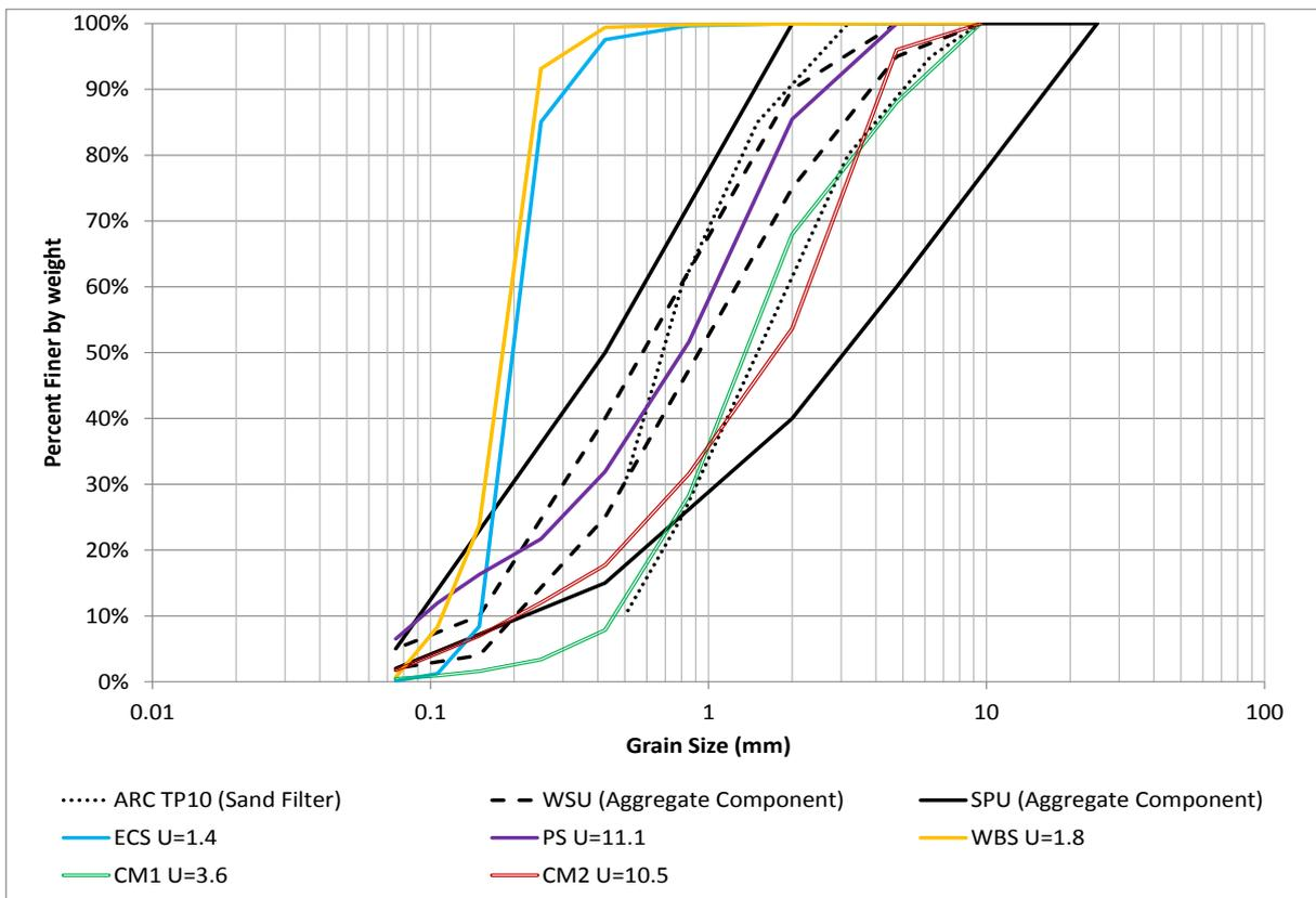
Figure 13a PSDs of aggregates sampled (non-cumulative bands)
