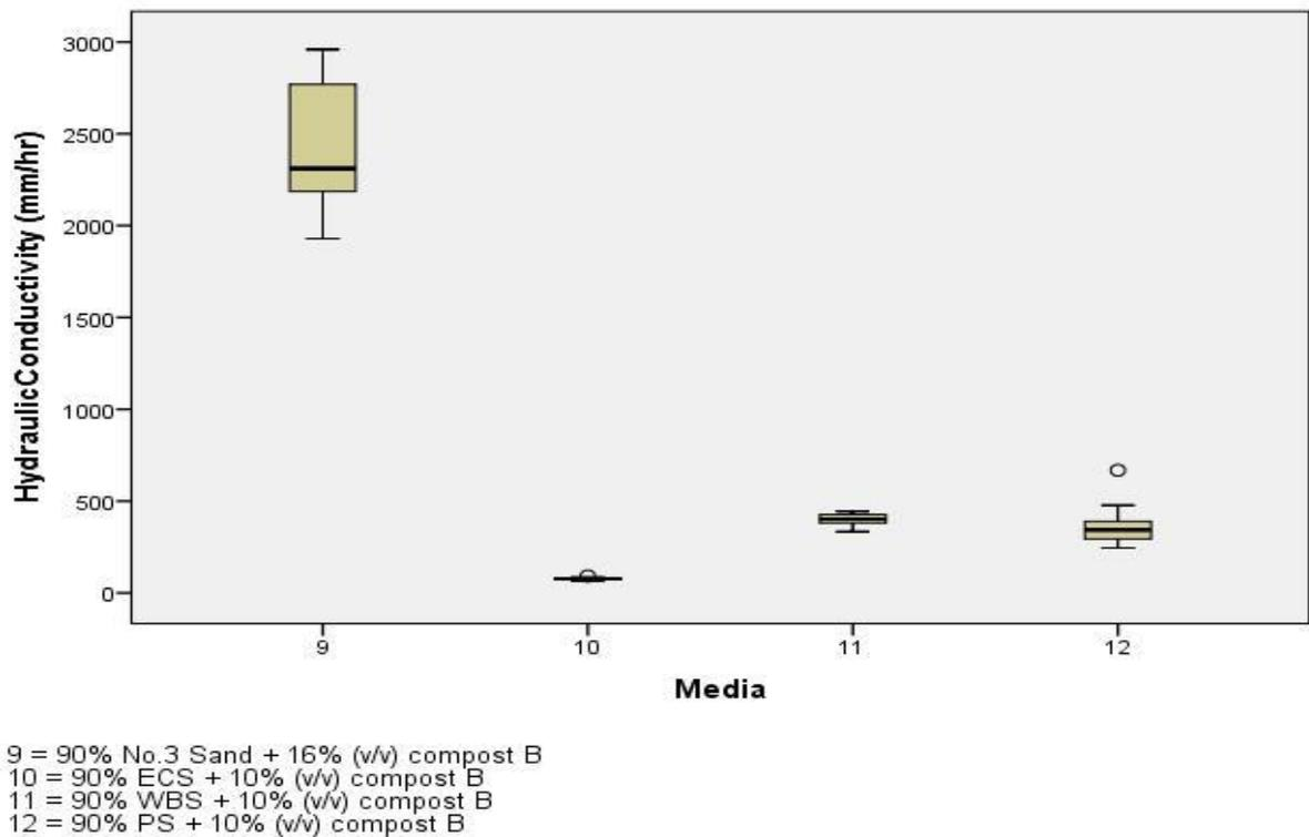
All three of the relatively “successful” sands have higher percentage fines than the recommended guidelines, while two out of three are poorly graded. All three have extremely different PSDs compared to the “best fitting” No.3 Sand. With this result, it is clear the PSD-based guidelines should not be used as a substitute to hydraulic conductivity testing.
