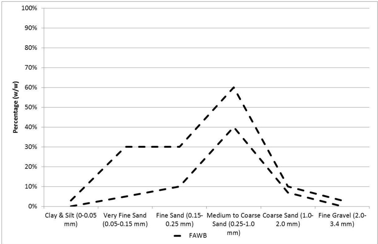
Figure 6 Compost PSD limits for candidate bioretention filter media according to Seattle Public Utilities (2008).
