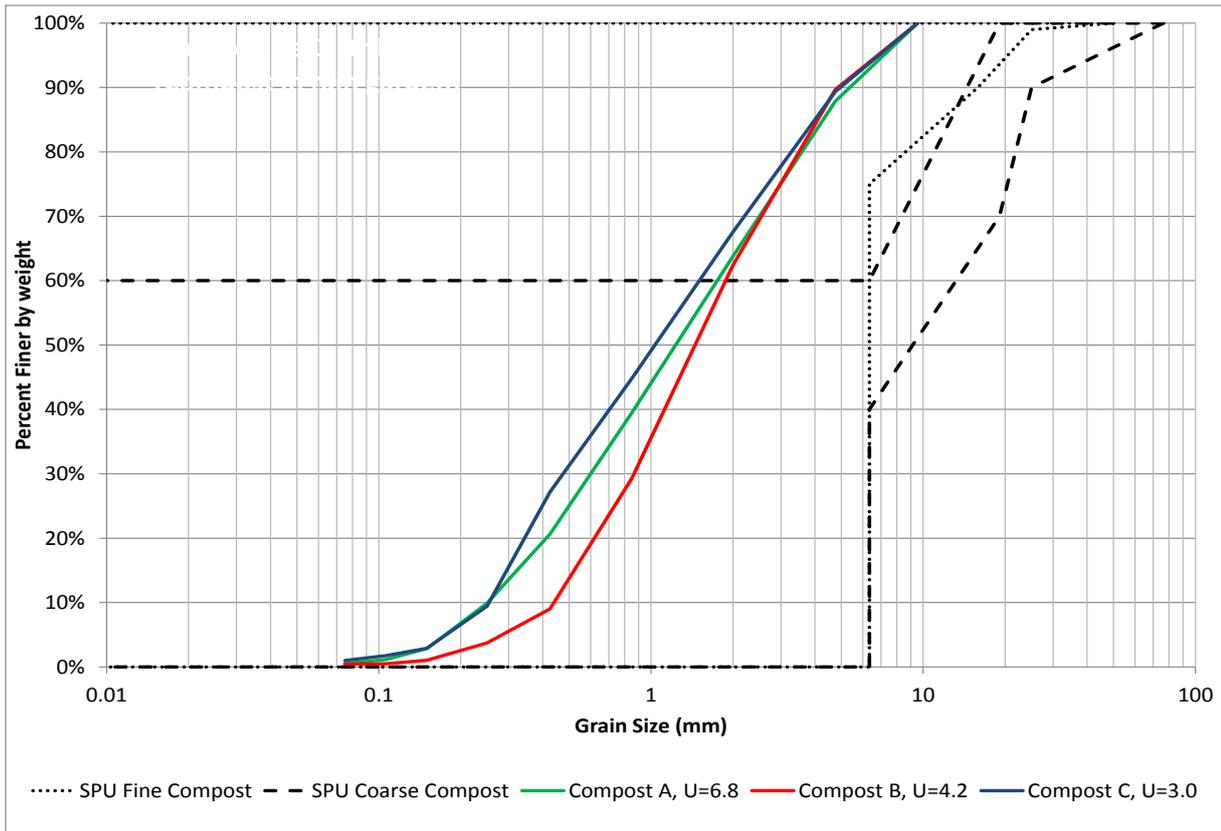
Figure 15 Variation in PSD of aggregates sampled three months apart
