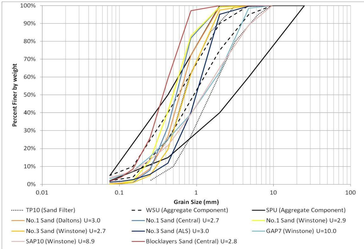
Figure 12b PSDs of aggregates sampled (cumulative limits)
