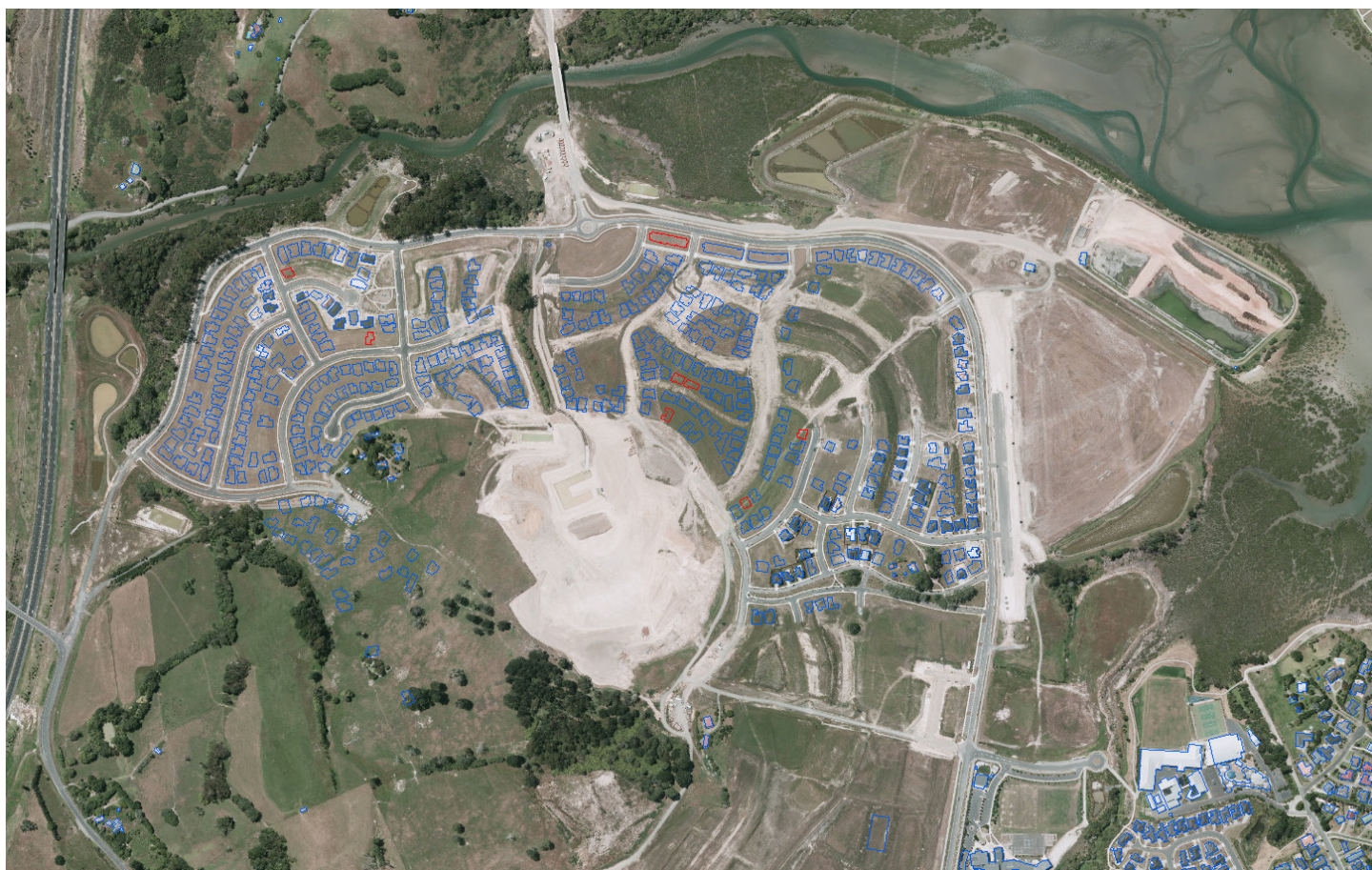
The 2013 building footprint layer captures new construction since 2010 and buildings not previously captured. Here: the Millwater development between SH1 and the Whangaparaoa Peninsula (overlaid on 2010 aerial photography) showing 2013 outlines (blue – existing buildings; red – under construction).
