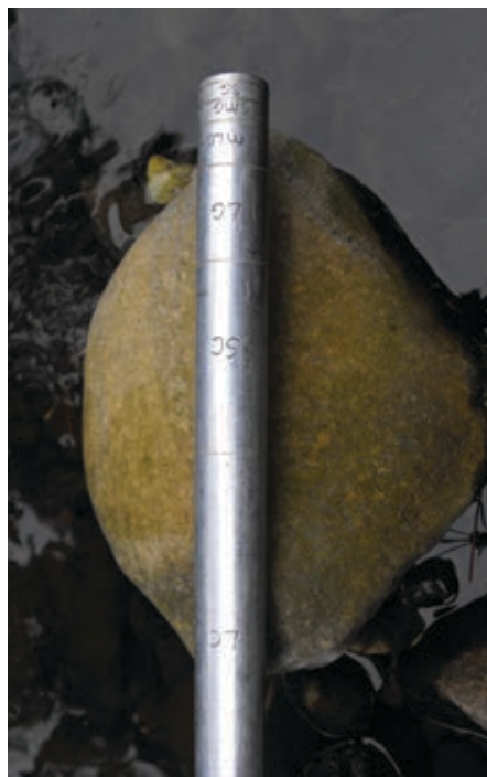
Fig. 7 Measuring a medium-large gravel particle (16 to 32mm) using the Wolman stick
