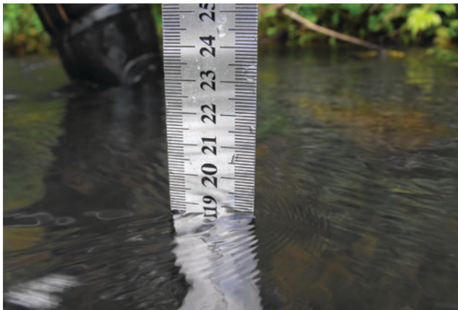
Fig. 22 Moderate velocity; difference (d_2-d_1) = 12\text{mm}
