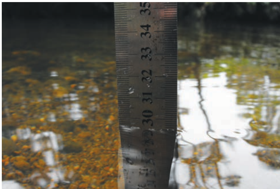
Fig. 20 Slow velocity; difference ( d_2 - d_1 ) = 1mm, so use floating particle test
