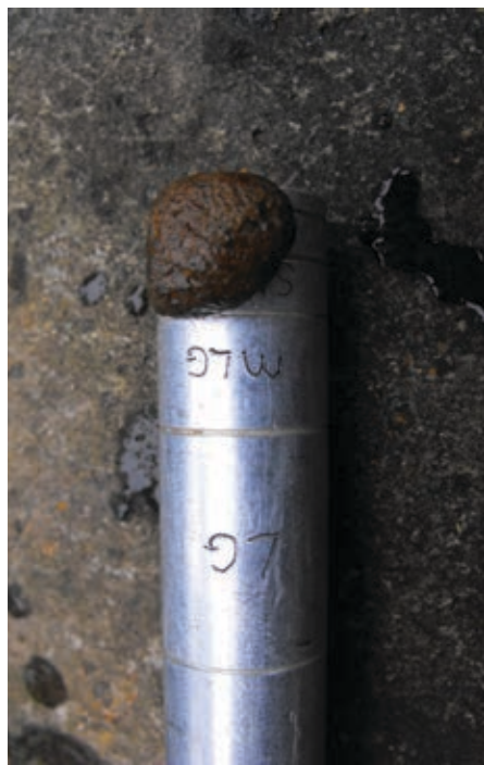
Fig. 7 Measuring a medium-large gravel particle (16 to 32mm) using the Wolman stick
