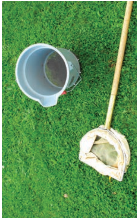
Fig. 4 Kick net and sieve bucket
