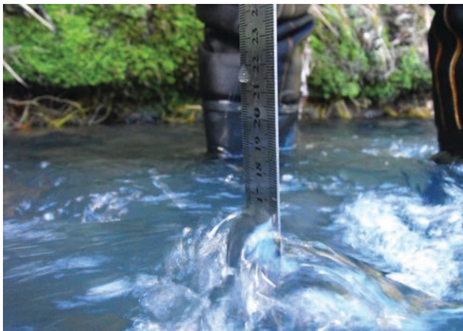
Fig. 25 Swift velocity; difference( d_2-d_1 ) = 53mm
