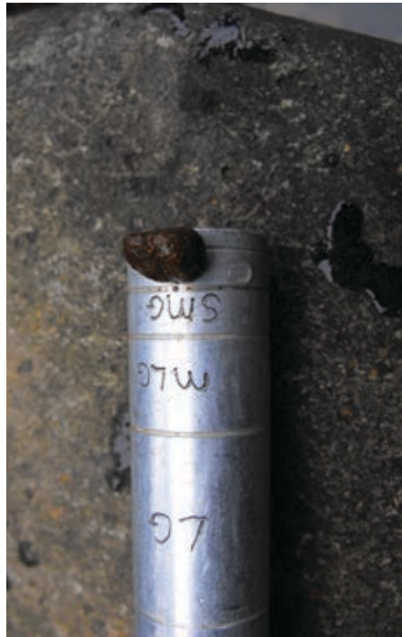
Fig. 6 Measuring a small gravel particle (2 to 8mm) using the Wolman stick
