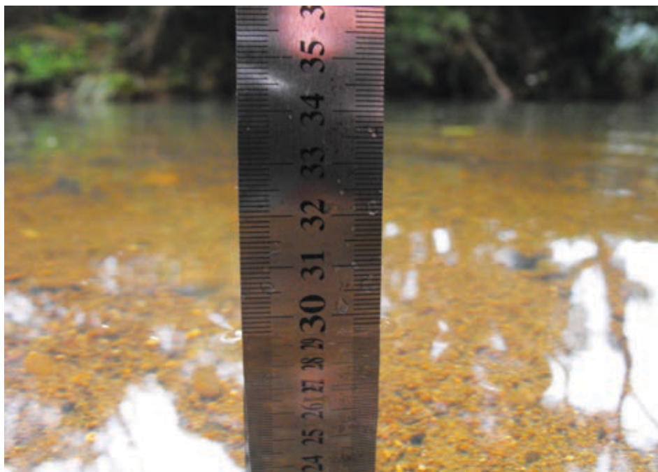
Fig. 21 Slow velocity; difference ( d_2 - d_1 ) = 1mm, so use floating particle test
