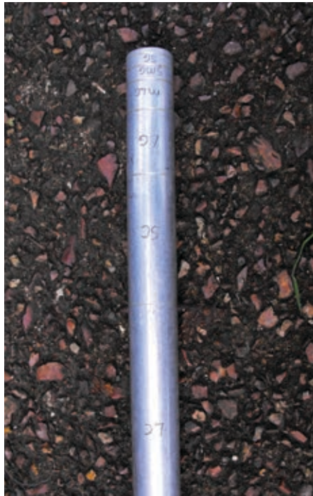
Fig. 2 Wolman (particle size) stick
