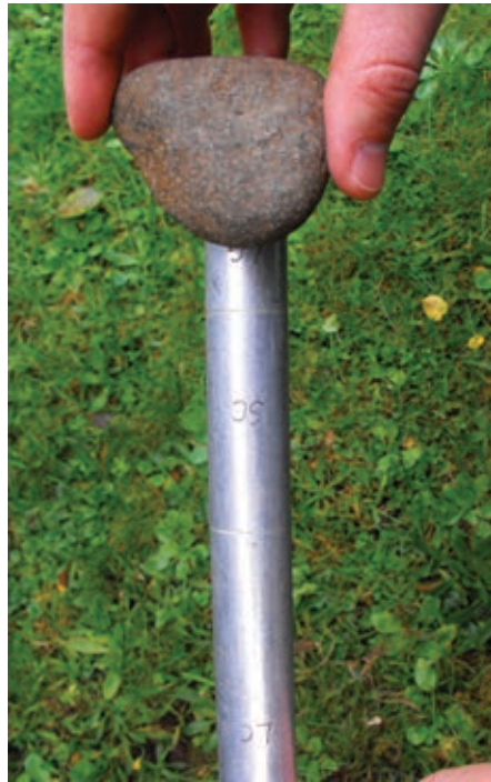
Fig. 8 Measuring a large gravel particle (32 to 64mm) using the Wolman stick
