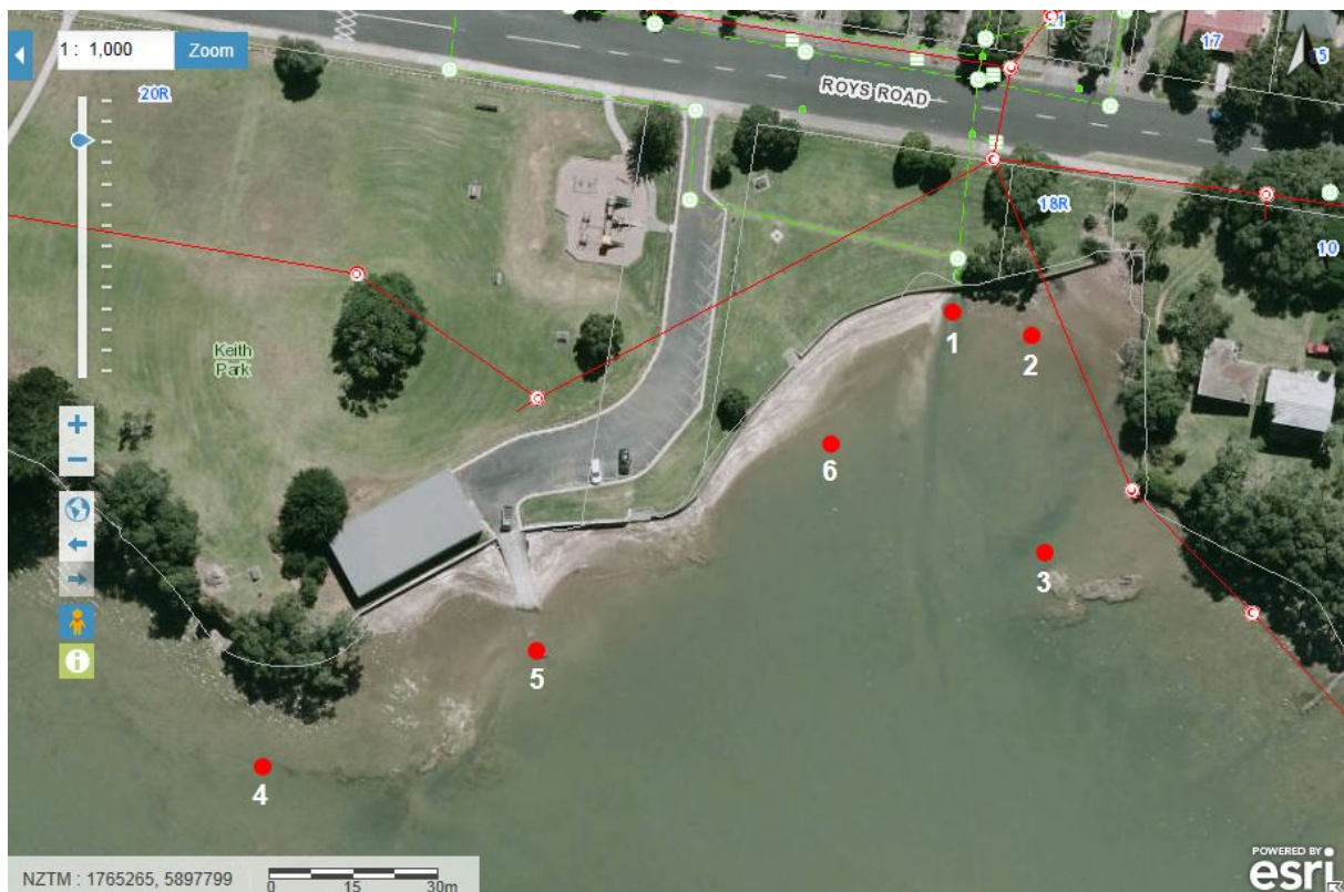
Figure 2-1 Location of 6 sampling sites visited during this investigation in 2014 (red dots). Stormwater lines and manholes are shown by green lines and green and white dots, respectively. Wastewater lines and manholes are shown with red lines and red and white dots, respectively.
